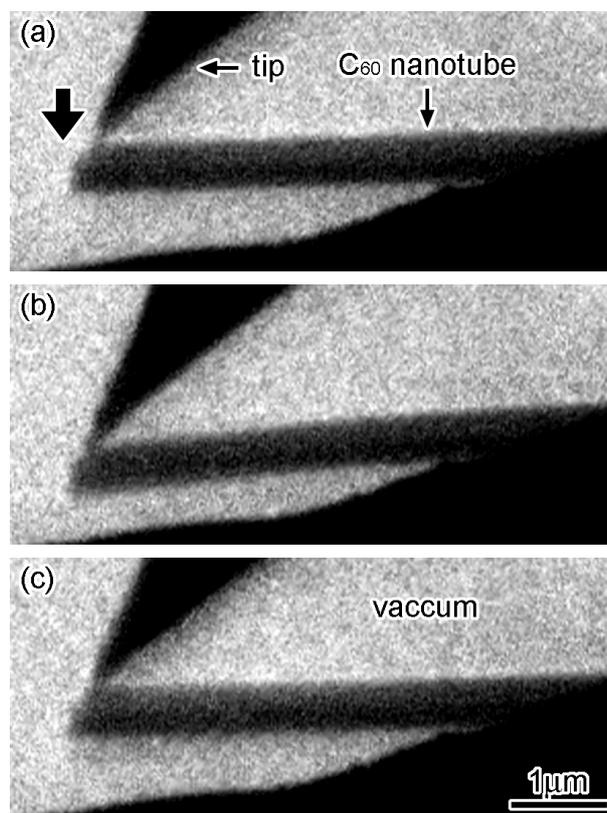
Fig. 2 (a) - (c) Time-sequential images of bending deformation of C<sub>60</sub> nanotube as observed in Fig. 1. The effective length for bending is  $4.8 \pm 0.2 \mu\text{m}$ .
