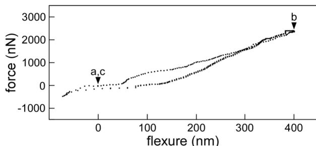
Fig. 3 Flexure - force curve of nanotube during bending observed in Fig. 2. The points indicated by arrowheads a-c correspond to the TEM images in Fig. 2 (a) - (c).
