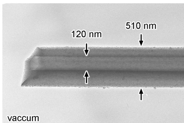
Fig. 1 TEM image of C<sub>60</sub> nanotube. The outer diameter is 510 nm and the inner diameter is 120 nm.
