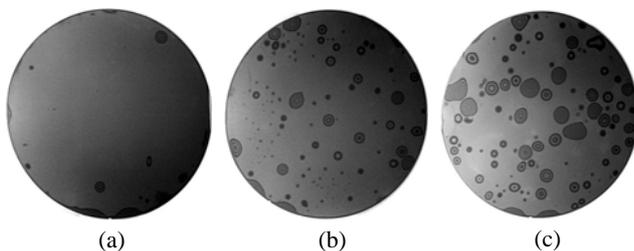
Fig. 3 IR transmission images of samples A (a), B (b) and C (c) after annealing at 800°C for 7 h, respectively
