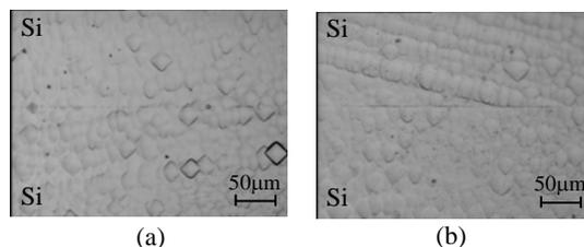
Fig. 5 Bonded interfaces of the sample D after KOH etching (a) before (b) after annealing at 700 °C for 2 h
