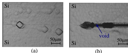
Fig. 6 Bonded interfaces of the sample E after KOH etching (a) before (b) after annealing at 700 °C for 2 h
