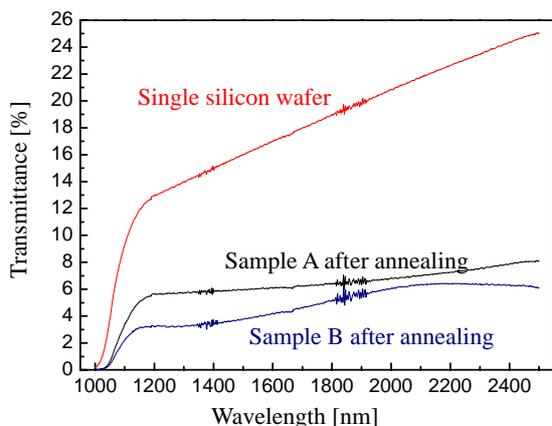
Fig. 4 Transmittance of the bonded wafer samples after annealing at 800°C and single silicon wafer as a reference
