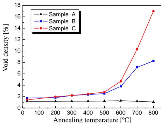
Fig. 2 Evolution of void densities as a function of annealing temperatures for the bonded wafers
