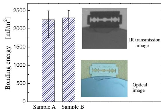
Fig. 1 Bonding energies of sample A (pretreated by O<sub>2</sub> RIE 10 s + N<sub>2</sub> radicals 60 s) and B (pretreated by O<sub>2</sub> RIE 60 s + N<sub>2</sub> radicals 60 s), the sample A was broken by inserting razor blade (right images) as an example
