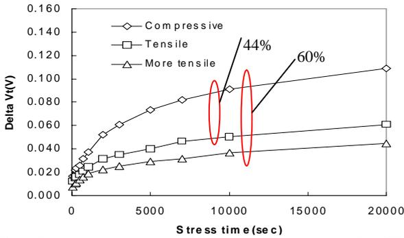
Fig.1 Delta  $V_t$  vs stress time under 125degree C and various SiN CESL stress.
