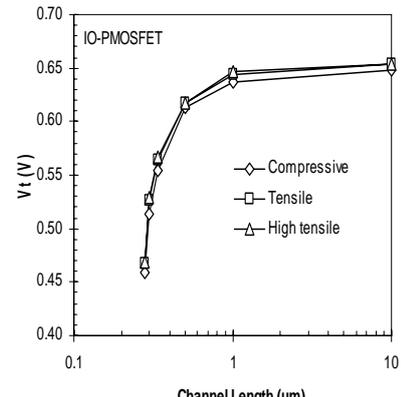
Fig. 6 IO-PMOSFET  $V_t$  vs channel length in Dual gate Oxide process.
