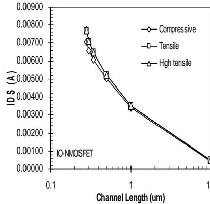
Fig. 3 IO-NMOSFET  $I_{DS}$  vs channel length in Dual gate Oxide process.
