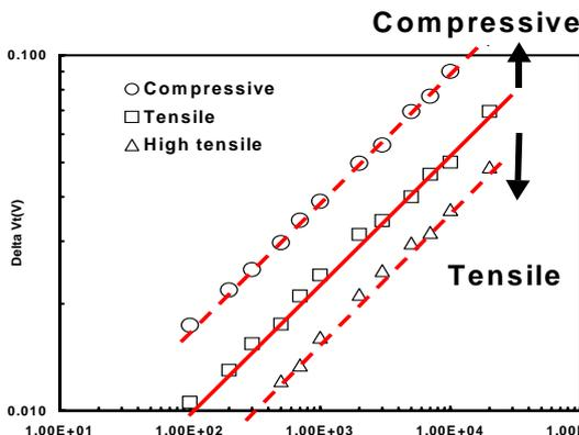
Fig.2 Delta  $V_t$  vs stress time under 125degree C and various SiN CESL stress (log-log plat).
