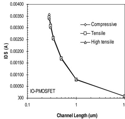
Fig. 5 IO-PMOSFET  $I_{DS}$  vs channel length in Dual gate Oxide process.
