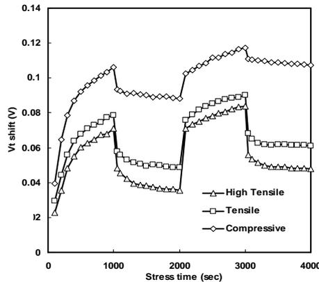
Fig. 7 Delta  $V_t$  vs stress time under the dynamic NBTI test with various stress for dual gate oxide I/O pMOSFET.
