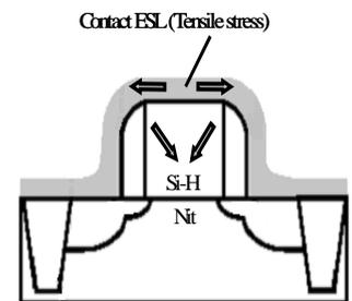
Fig. 8 The Si-H bonds are harder to dissociate and easier to bond for tensile stress film
