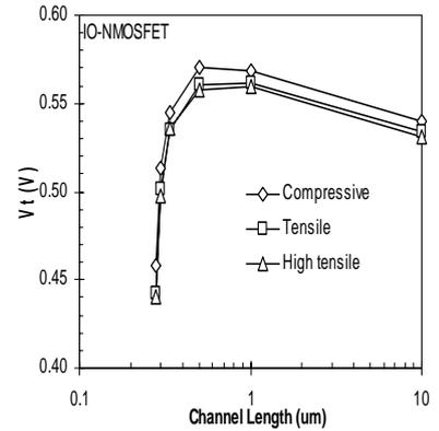
Fig. 4 IO-NMOSFET  $V_t$  vs channel length in Dual gate Oxide process.
