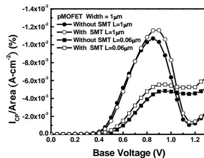
Figure 6: Charge-pumping current versus base voltage for pMOSFET with and without SMT. Comparison was made for long channel and short channel devices.
