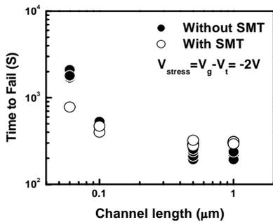
Figure 5: NBTI lifetime comparison for samples with and without SMT. Comparison was made for different channel lengths. Measurement was performed at 125°C.
