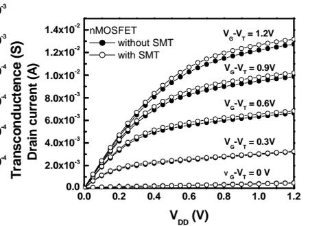
Figure 3: Comparison of  $I_d$ - $V_d$  to show the difference for nMOSFET with and without SMT.
