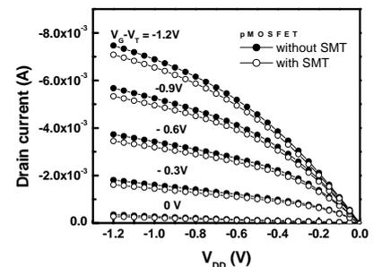
Figure 4: Comparison of  $I_d$ - $V_d$  to show the difference for nMOSFET with and without SMT.
