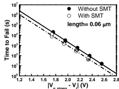
Figure 8: Comparison of NBTI lifetime for short channel devices with and without SMT. Introduction of SMT degrades NBTI by 2-3 times (Temperature=125°C, channel length=0.06μm)
