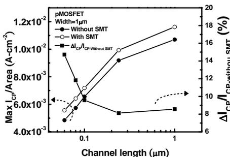
Figure 7: Maximum charge pumping current as function of channel length. The difference (comparing with SMT to without SMT) in charge-pumping current becomes more evident for shorter channel length.
