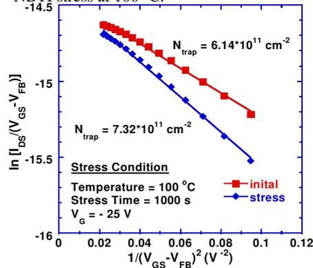
Fig. 4 Grain-boundary trap-state density extraction of the LTPS TFT.
