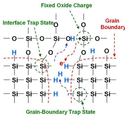
Fig. 9 Schematic diagram illustrating the NBTI degradation in LTPS TFTs.
