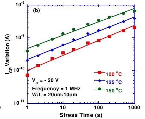
Fig. 7 Time dependence of  $\Delta I_{CP}$  with various (a) stress voltages and (b) stress temperatures.
