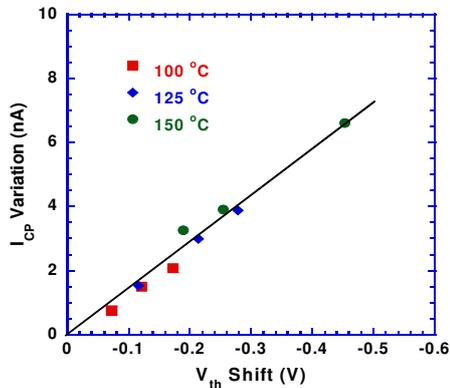
Fig. 8 Correlation between  $\Delta I_{CP}$  and  $\Delta V_{th}$ .
