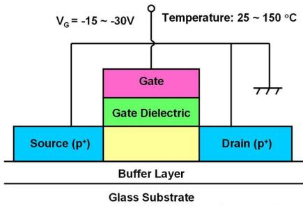
Fig. 1 Schematic cross-sectional view of the LTPS TFT and the stress setup.
