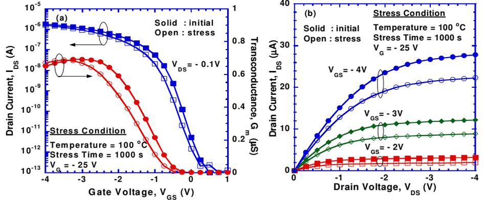
Fig. 2 (a) Transfer and (b) output characteristics of the LTPS TFT before and after 1000-s NBTI stress at 100 °C.
