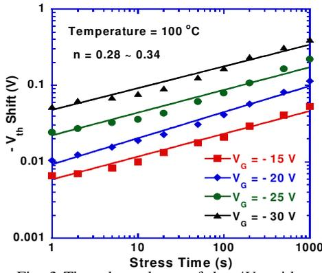
Fig. 3 Time dependence of the  $\Delta V_{th}$  with various stress voltages at 100 °C.
