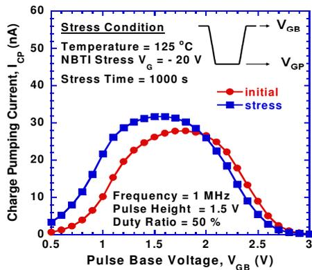
Fig. 6 Charge-pumping current before and after NBTI stress at 125 °C.
