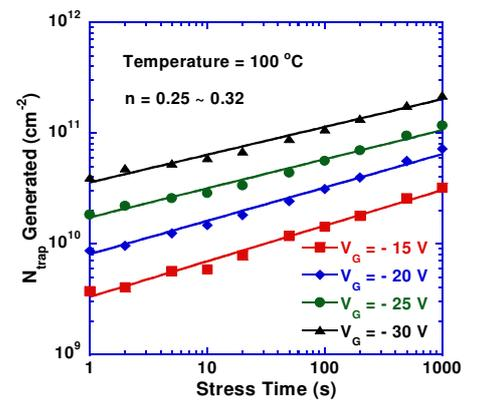
Fig. 5 Time dependence of the  $\Delta N_{trap}$  with various stress voltages at 100 °C.
