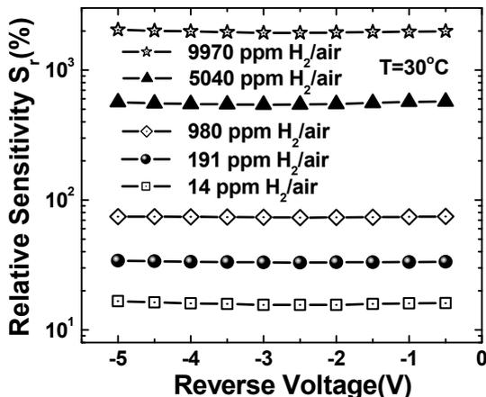
Fig. 4 Relationship between the relative sensitivity ratio  $S_r(\%)$  and reverse bias under different hydrogen concentrations at 30°C
