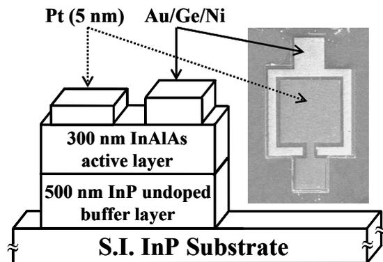
Fig. 1 Schematic cross section and SEM picture of the studied 5-nm-Pt/In<sub>0.52</sub>Al<sub>0.48</sub>As Schottky diode-type hydrogen sensor.
