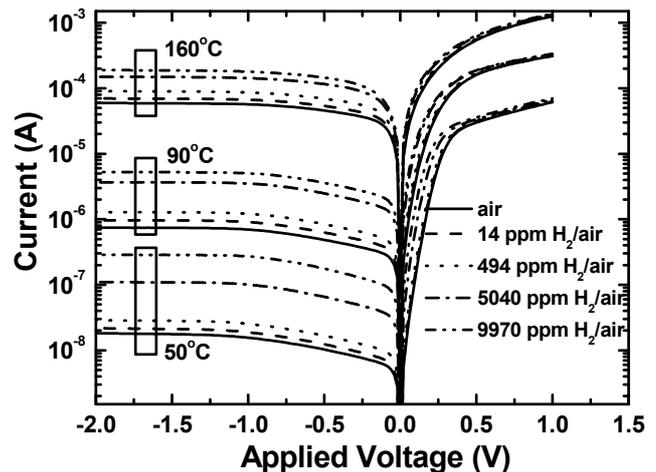
Fig. 2 Measured I-V characteristic curves of the studied 5-nm-Pt/In<sub>0.52</sub>Al<sub>0.48</sub>As MS Schottky diode under different concentrations of hydrogen gases at 50, 90, and 160°C, respectively.
