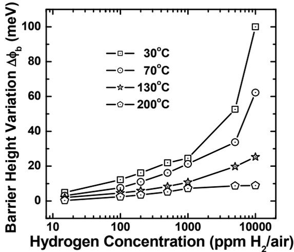
Fig. 3 Schottky barrier height variation ( $\Delta\phi_b$ ) as a function of temperature with various hydrogen concentrations ranging from 14 to 9970 ppm  $H_2$ /air.
