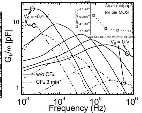
Fig. 8. Frequency dependent conductance  $G_p/\omega$  for a series of gate voltage for forming gas annealed samples without CF<sub>4</sub> plasma treatment and samples with CF<sub>4</sub> plasma treatment for 3 min. Inset is the extracted midgap  $D_{it}$ .
