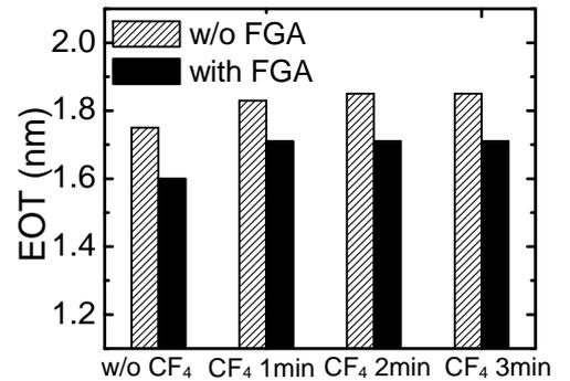
Fig. 5. Equivalent oxide thickness (EOT) for samples both with and without FGA of different CF<sub>4</sub> treatment conditions.
