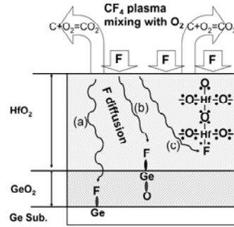
Fig. 1. F incorporation into high-k/Ge gate stack and various possible passivation mechanisms during subsequent annealing steps: (a) passivation of interface traps at GeO<sub>2</sub>/Ge interface; (b) passivation of interface traps at HfO<sub>2</sub>/GeO<sub>2</sub> interface; (c) passivation of HfO<sub>2</sub> bulk traps.
