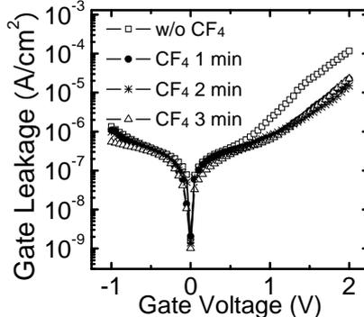
Fig. 7.  $I_g$ - $V_g$  characteristics for forming gas annealed samples with different CF<sub>4</sub> plasma treatment conditions.
