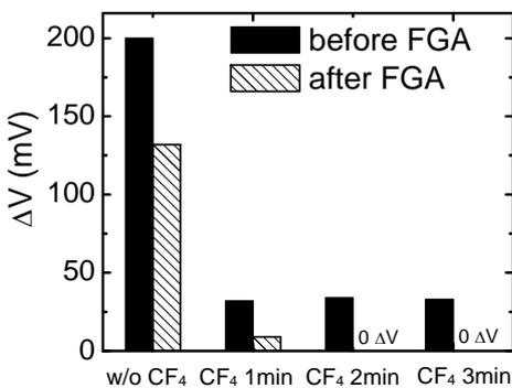
Fig. 6. Frequency dependent flat band voltage shifts ( $\Delta V$ ) for samples both with and without FGA of different CF<sub>4</sub> treatment conditions.
