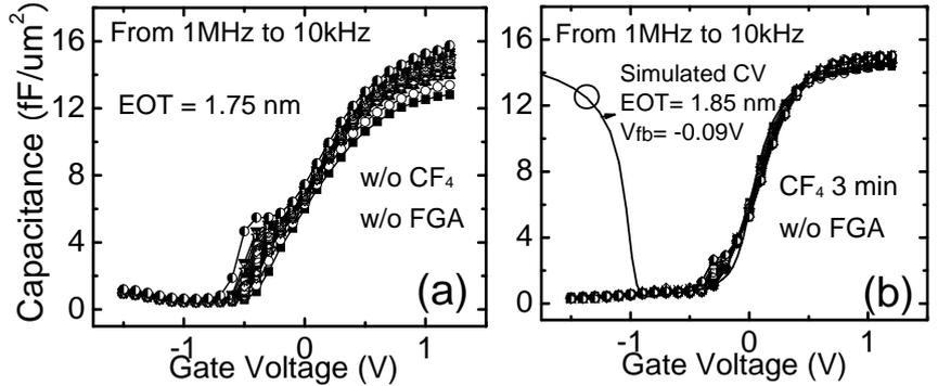
Fig. 3. Capacitance-voltage characteristics of TaN/HfO<sub>2</sub>/GeO<sub>2</sub>/Ge gate stacks (~ 2 nm GeO<sub>2</sub> and 4.5 nm HfO<sub>2</sub>) without FGA measured at 1MHz, 900kHz, 800kHz, ..., 200kHz, 100kHz, 90kHz, 80kHz, ..., 20kHz and 10kHz (a) without CF<sub>4</sub> plasma treatment and (b) with CF<sub>4</sub> plasma treatment for 3 min.
