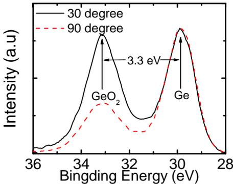
Fig. 2. Angle resolved XPS Ge 3d spectra for germanium samples after the thermal oxidation at 400°C. The thickness of GeO<sub>2</sub> is about 2 nm.
