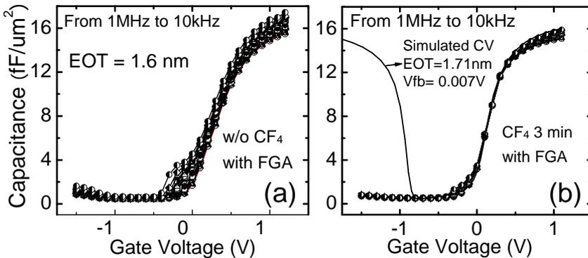
Fig. 4. Capacitance-voltage characteristics of TaN/HfO<sub>2</sub>/GeO<sub>2</sub>/Ge gate stacks (~ 2 nm GeO<sub>2</sub> and 4.5 nm HfO<sub>2</sub>) with FGA at 350°C for 1 hour measured at 1MHz, 900kHz, 800kHz, ..., 200kHz, 100kHz, 90kHz, 80kHz, ..., 20kHz and 10kHz (a) without CF<sub>4</sub> plasma treatment and (b) with CF<sub>4</sub> plasma treatment for 3 min.
