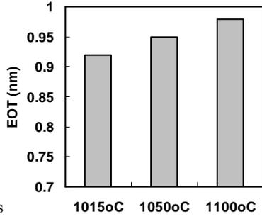
Fig. 1 EOT of the samples. (using CVC) RTA causes a slight EOT increase.
