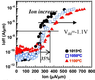
Fig. 4  $I_{on}$ - $I_{off}$  characteristics of pMOSFETs. With the effect of higher temperature RTA, Ion was increased.
