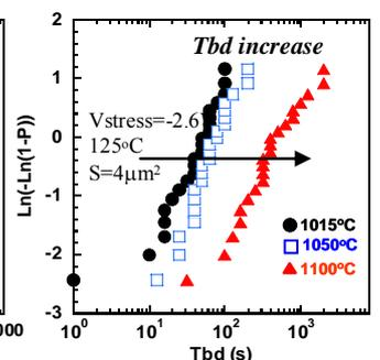
Fig. 10 Weibull distribution of  $T_{bd}$  of HfSiON. With RTA temperature increase,  $T_{bd}$  were increased.
