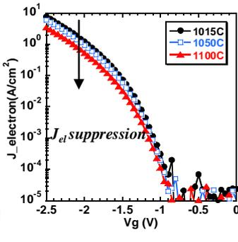
Fig. 12 Cathode injection electron as a function of gate bias. With RTA temperature increase, electron currents were suppressed.
