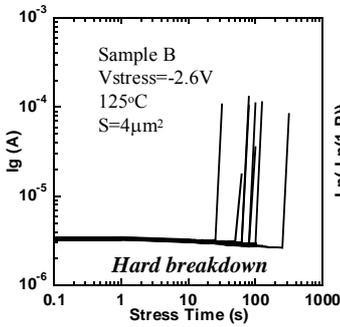
Fig. 9  $I_g$ - $t$  characteristics of Sample B. Abrupt gate leakage current jumps were observed.
