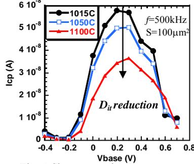
Fig. 5 Charge pumping current as a function of  $V_{base}$ . With RTA temperature increase,  $D_{it}$  values were decreased.
