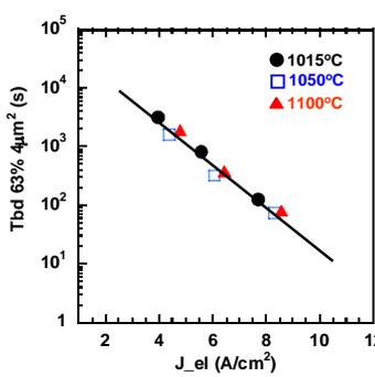
Fig. 13  $T_{bd}$  as a function of cathode injection electron. There exist a common relationship between  $T_{bd}$  and  $J_{el}$ .
