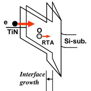
Fig. 14 Schematic of high temperature annealing. Oxygen in HfSiON oxidized Si substrate during RTA.
