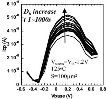
Fig. 7 Charge pumping current as a function of  $V_{base}$ . values were increased.
