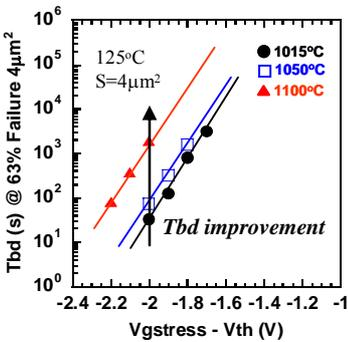
Fig. 11  $T_{bd}$  as a function of overdrive stress voltage. With RTA temperature increase, TDDB lifetimes were increased.
