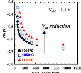
Fig. 2  $V_{th}$  as a function of gate length of pMOSFETs. Higher temperature RTA is effective for  $V_{th}$  reduction.
