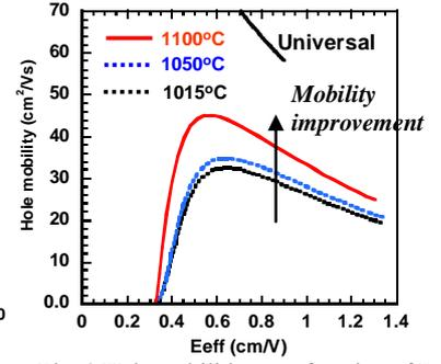
Fig. 3 Hole mobilities as a function of  $E_{eff}$ . With RTA temperature increase, mobilities were increased.
