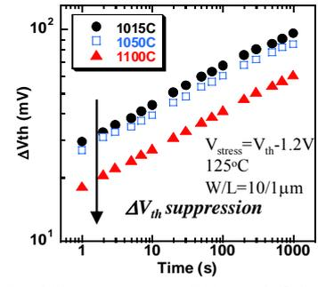
Fig. 6 Time evolution of  $\Delta V_{th}$  in NBTI. With RTA temperature increase,  $\Delta V_{th}$  were suppressed.
