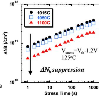
Fig. 8 Time evolution of  $\Delta N_{it}$ . With RTA temperature increase,  $\Delta N_{it}$  were suppressed.
