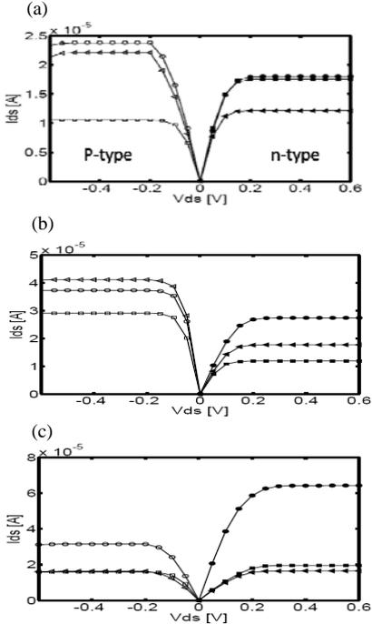
Fig. 3:  $I_{ds} - V_{ds}$  curves for (a) Si, (b) Ge and (c) GaAs NW FETs. The gate oxide thickness is 1.6nm and the off-current is set to 60nA at  $V_{dd}=0.6V$ . Square Symbols for [100] orientation, Circle Symbols for [110] orientation and Triangle Symbols for [111] orientation. For n-type device, the highest on-current is given by [110] channel orientation in all materials, while for p-type, the highest on-current is given by [110], [111] and [110] in Si, Ge, and GaAs cases, respectively.
