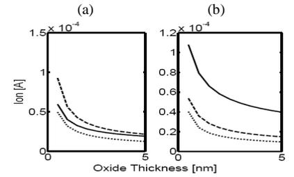
Fig. 9: Ion-oxide thickness curves for Si, Ge and GaAs for (a) p-type and (b) n-type. GaAs has overall high on-current for n-type while Ge for p-type.
