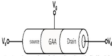
Fig. 1: A schematic of the simulated Cylindrical Nanowire FETs. The diameter of the Circular cross-section ( $D$ ) is 3nm. The oxide thicknesses ( $tox$ ) for this simulation are 0.5nm and 1.6nm.
