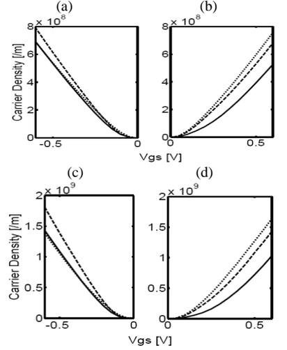
Fig. 7: Comparison of carrier density for Si (dotted line), Ge (dashed) and GaAs (solid line) NW FETs for  $tox=1.6nm$  for (a) n-type and (b) p-type and  $tox=0.5nm$  for (c) p-type and (d) n-type. Si has the largest electron density but Ge have the largest hole density.
