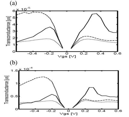
Fig. 8: Transconductance, gm curves for Si, Ge and GaAs NW FETs at (a)  $tox=1.6nm$  and (b)  $tox=0.5nm$  show Ge and GaAs give high gm, which agrees with high ON-current.
