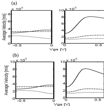
Fig. 6: Average velocity for Si (dotted line), Ge (dashed line) and GaAs (solid line) NW FETs for  $tox=1.6nm$  (a) and  $tox=0.5nm$  (b). GaAs has the highest electron average velocity while GaAs and Ge have similar hole average velocity.
