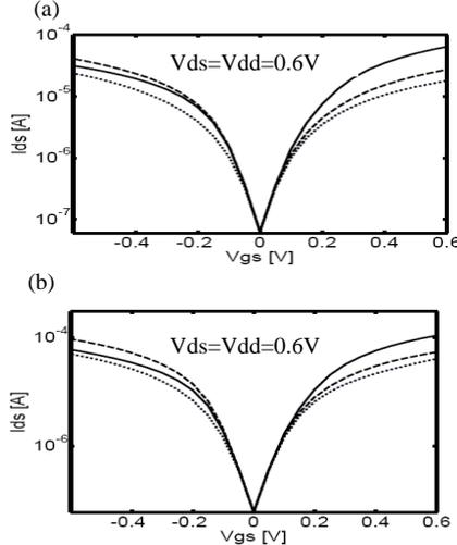
Fig. 5: Comparison of  $I_{ds} - V_{gs}$  curves for Si (dotted line), Ge (dashed line) and GaAs (solid line) NW FETs at (a)  $tox=1.6nm$  and (b)  $tox=0.5nm$ .
