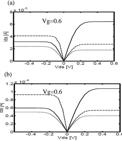
Fig. 4:  $I_{ds} - V_{ds}$  curves for Si (dotted line), Ge (dashed line) and GaAs (solid line) NW FETs at (a)  $tox=1.6nm$  and (b)  $tox=0.5nm$ . Ge NW FET outperforms the other two cases for p-type MOFETs while GaAs NW MOSFET outperforms the other cases for n-type MOSFETs.
