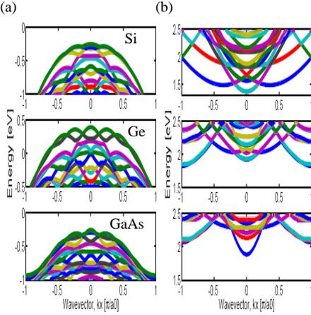
Fig. 2: (a) and (b) Simulated E-k diagram of valence and conduction band for channel orientation [100], respectively, for Si, Ge and GaAs using sp3d5s\* empirical TB model.
