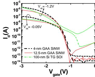
Fig. 4:  $I_d$ - $V_g$  characteristics of three devices on a single wafer: a 4-nm and a 12.5-nm diameter GAA SiNW and a 1- $\mu$ m width, 100-nm Si body SOI top-gated planar device. Device parameters are shown in Table 1.
