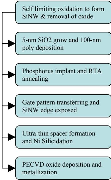
Fig. 1: Process flow of the GAA SiNW NiSi Schottky barrier MOSFETs
