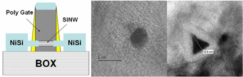
Fig. 2: (a) estimated final device structure of GAA SiNW NiSi SB-MOSFET, with NiSi encroached through the thin spacer ( $< 25$ -nm). (b) TEM image of a 4-nm diameter SiNW cross section. (c) TEM image of a 12.5-nm width SiNW cross section. Gate oxide thickness is  $\sim 5$ nm.
