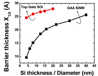
Fig.8: Calculated Full-Barrier-Width at Half Maximum ( $X_{1/2}$ ) as a function of the Si body thickness of top-gated SOI planar devices and GAA SiNW diameters.
