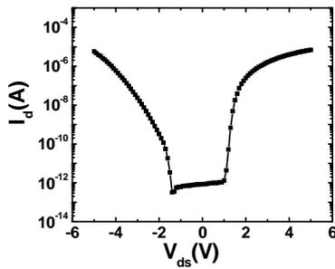
Fig. 3: Current-Voltage characteristics of a 12.5-nm GAA SiNW at zero gate bias. The total resistance obtained at large gate bias is  $0.3486 \text{ M}\Omega$  and the fitted carrier density is  $7.26\text{E}18 \text{ cm}^{-3}$  according to the method in reference 5.
