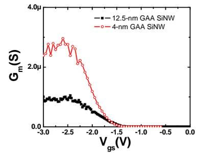
Fig.5: The transconductance of the 4-nm-diameter and 12.5-nm-diameter GAA SiNW in Fig. 4. Both increases as gate bias increases negatively and become a constant when gate bias is negatively larger than certain value.
