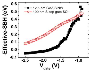
Fig.6: Effective-SBH of the 12.5-nm diameter GAA SiNW and the 1- $\mu$ m width, 100-nm Si top-gated SOI planar SBFET as a function of gate bias.
