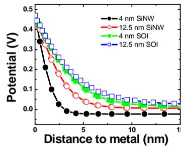
Fig.7: Calculated potential profile of the SB at on-state. The circle ones represent the GAA SiNW and the square ones represent top-gated SOI SBFET.
