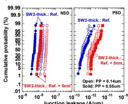
Fig. 16. Distribution of poly bounded silicide junction for minimum and large poly pitch.
