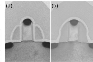
Fig. 6. TEM cross-section of NFETs with different SW2 structures. (a)  $Si_3N_4/SiO_2$  stack and (b)  $Si_3N_4$ -only structures, respectively.
