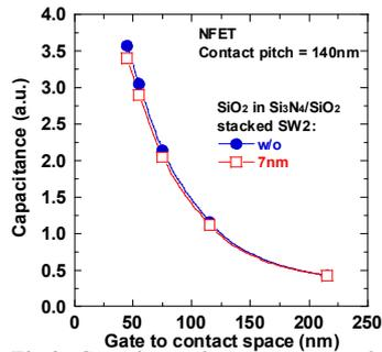
Fig. 8. Capacitance between gate and contact with and without  $SiO_2$  in SW2 stack.
