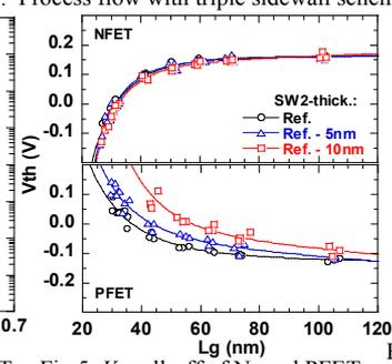
Fig. 5.  $V_{th}$  roll-off of N- and PFETs with different SW2 deposition thickness.
