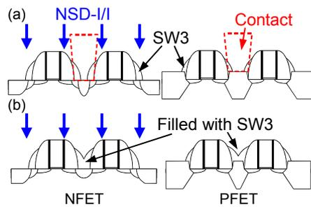
Fig. 13. Schematic diagram of SW3 design to achieve minimum (a) contacted and (b) non-contacted poly pitch.
