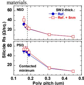
Fig. 15. Poly bounded silicide sheet resistance as a function of poly pitch.
