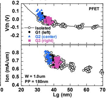
Fig. 18. PFET  $V_{th}$  and  $I_{on}$  vs.  $L_g$  for three-stacked layout with min. contacted poly pitch.
