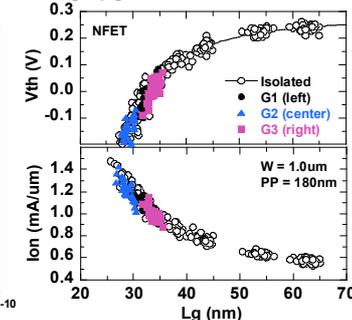
Fig. 17. NFET  $V_{th}$  and  $I_{on}$  vs.  $L_g$  for three-stacked layout with min. contacted poly pitch.
