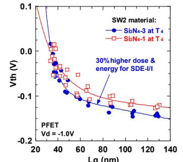
Fig. 11. Comparison of PFET  $V_{th}$  roll-off for different SW2- $Si_3N_4$  materials.
