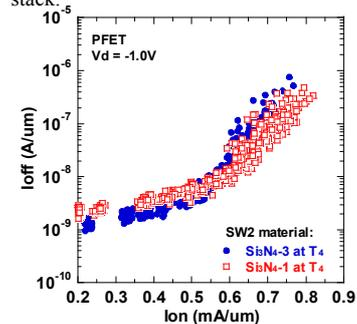
Fig. 12. Comparison of PFET  $I_{on}$ - $I_{off}$  characteristics for different SW2- $Si_3N_4$  materials.
