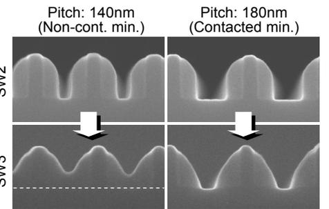
Fig. 14. SEM cross-section of NFET after SW2 and SW3 formation for two different poly pitches (140/180nm).
