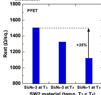
Fig. 9. Comparison of PFET  $R_{ext}$  for different SW2- $Si_3N_4$  materials.
