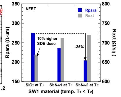
Fig. 3. Comparison of NFET  $R_{para}$  and  $R_{ext}$  for different SW1 materials.
