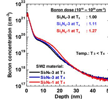
Fig. 10. SIMS profiles of PFET SDE for different SW2- $Si_3N_4$  materials.
