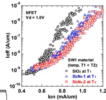
Fig. 2. Comparison of NFET  $I_{on}$ - $I_{off}$  characteristics for different SW1 materials.
