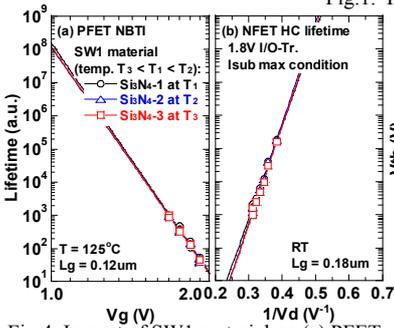
Fig. 4. Impact of SW1 material on (a) PFET NBTI and (b) NFET HC lifetime.
