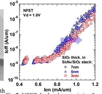
Fig. 7. NFET  $I_{on}$ - $I_{off}$  characteristics for different  $SiO_2$  thickness in SW2 stack.
