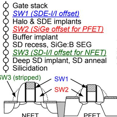
Fig. 1. Process flow with triple sidewall scheme.
