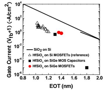
Fig.3 Gate leakage current density ( $J_g$ ) of HfSiO<sub>2</sub> dielectric on SiGe channel pMOSFETs. ( $\sim 3 \times 10^2$  lower than SiO<sub>2</sub>/Si channel) at EOT of 14Å.
