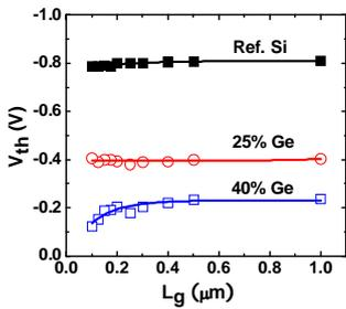
Fig.4 Low  $V_{th}$  of -0.41V (25% Ge) and -0.24V (40% Ge) of SiGe channel pMOSFETs, which are significantly lower than  $V_{th}$  of ref. Si channel.
