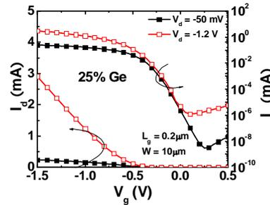
Fig.8 Well behaved short channel  $I_d$ - $V_g$  of SiGe channel pMOSFETs (25% and 40% Ge).
