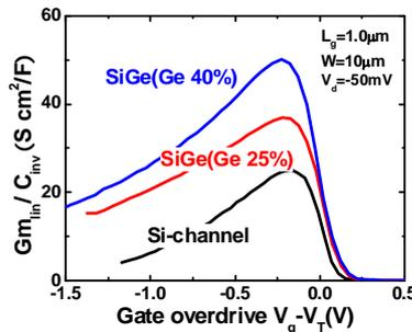
Fig.11 Normalized  $G_m$  of SiGe channels over universal SiO<sub>2</sub>/Si channel and optimized high-k dielectric/metal gate Si channel.
