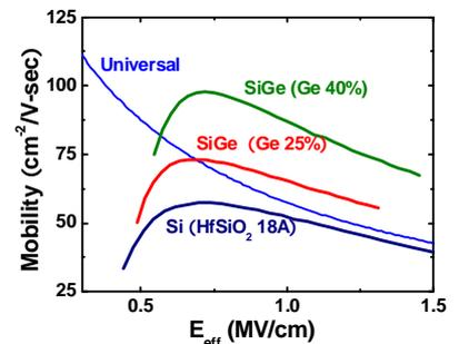
Fig.12 A mobility enhancement of 50% and 13% from 40% and 25% SiGe channel pMOSFETs, respectively, over universal mobility.
