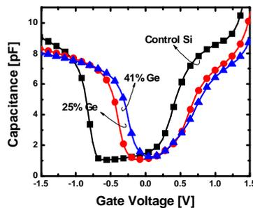
Fig.10 Measured C-V exhibit slightly high  $V_{th}$  and stretch-out for high Ge% due to higher  $Q_i$ .  $V_{th}$  shows an expected trend as simulation results.
