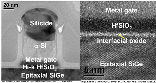
Fig.1 (a) Bright-field and (b) high-resolution XTEM images of gate stack with HfSiO<sub>2</sub> high-k gate dielectrics and metal gates fabricated on high-quality epitaxial SiGe layers selectively grown on Si (100) substrates using a CVD system.
