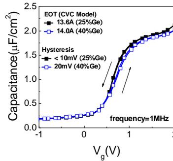
Fig.2 C-V of SiGe MOS capacitors with low EOT and minimal hysteresis. (40Å HfSiO<sub>2</sub>). Slightly higher C-V stretch-out observed with 40% Ge due to higher interface charge density.
