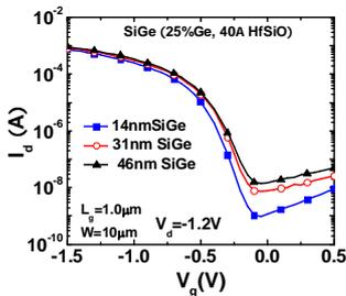
Fig.7 Improved GIDL and SS characteristics by reducing SiGe channel thicknesses due to relatively small SiGe portion in electrostatic field.
