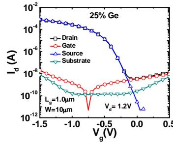
Fig.6 GIDL currents are governed either by gate leakage current (25% Ge) or substrate current (40% Ge), which confirms a high BTBT current on small band gap energy channel materials (or high Ge %).
