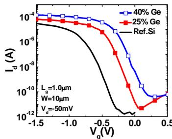
Fig.5 SS (70~78mV/dec) of SiGe channels comparable with ref. Si channel. GIDL, however, increases due to BTBT current when Ge % increases.
