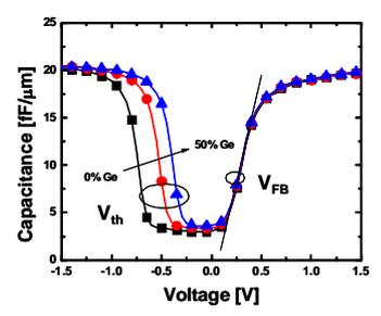
Fig.9 Simulated C-V shows identical  $V_{th}$  and varying  $V_{th}$  with increasing Ge% due to changes in depletion charge and surface potential.
