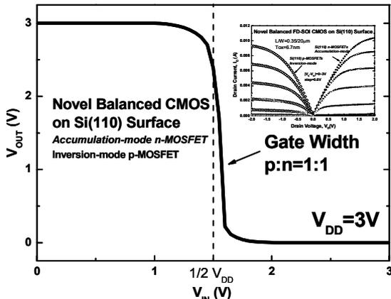
Fig. 6 The ideal  $V_{in}$ - $V_{out}$  characteristics of the novel balanced CMOS inverter with AM n-MOSFET and IM p-MOSFET on Si(110) for gate width ratios of pMOSFET/nMOSFET=1:1.
