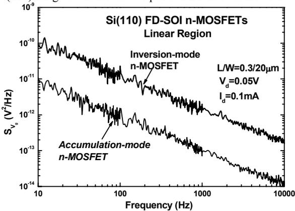
Fig. 8  $1/f$  noise level in AM n-MOSFETs operated at linear region on Si(110) is suppressed about 1 digit compared with that in IM n-MOSFET.
