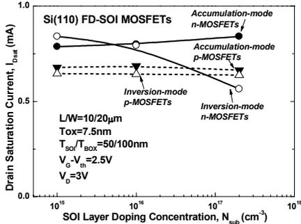
Fig. 3 Drain Saturation Current as a function of  $N_{sub}$  in n- and p-MOSFETs on Si(110).  $I_{Dsat}$  increases with increasing the  $N_{sub}$  in AM n-MOSFETs and shows no dependence on  $N_{sub}$  in p-MOSFETs.
