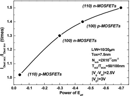
Fig. 5  $I_{dsat}$  improvement in AM MOSFETs on Si(100) and (110) as a function of the power of  $E_{eff}$ . This result indicates the mechanism for the current improvement in AM MOSFETs is resulted from the lowering  $E_{eff}$ .
