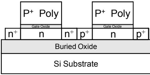
Fig. 1 Schematic of the novel balanced CMOS on Si(110) surface combined with AM n-MOSFET and IM p-MOSFET.
