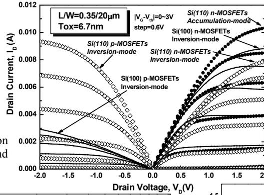
Fig. 2  $I_d$ - $V_d$  characteristics of n- and p-MOSFETs on Si(110) and (100) surfaces. A complete balanced CMOS is realized on Si(110) surfaces using AM n-MOSFET and IM p-MOSFET with very high current drivability. The current drivability of AM n-MOSFET on Si(110) is about 1.2 times larger than IM n-MOSFET on Si(100).
