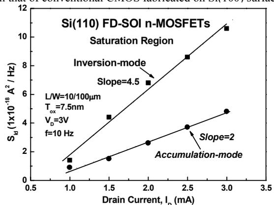
Fig. 9  $1/f$  noise levels in n-MOSFETs on Si(110) operated on saturation region as a function of drain current. The slope for AM n-MOSFETs is much smaller than that for IM n-MOSFETs.
