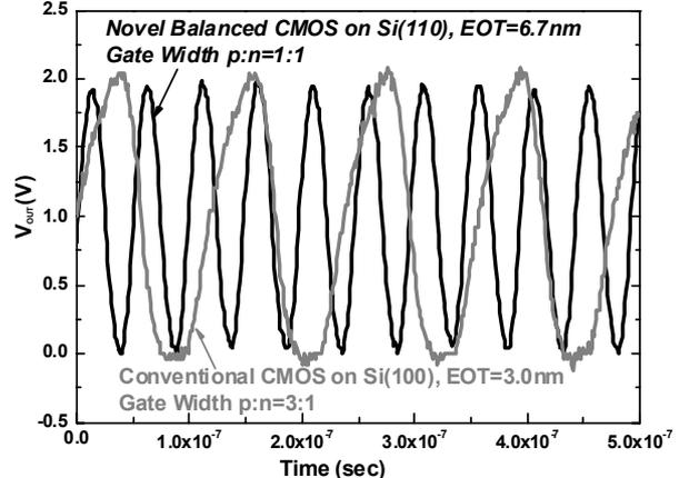
Fig. 7 The oscillation frequency of 101 stages of inverter chains for the same gate width in balanced CMOS on Si(110) is about 2 times higher than that of conventional CMOS fabricated on Si(100) surface.
