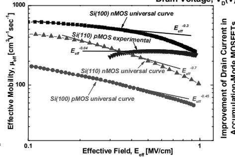
Fig. 4  $E_{eff}$ - $\mu_{eff}$  characteristics of electrons and holes on Si(100) and (110).  $\mu_{eff}$  in n-MOSFETs on Si(110) is expected to be improved most greatly by lowering  $E_{eff}$  and almost no improvement for holes on Si(110).
