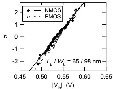
Fig. 2 Cumulative probability plot of  $V_{th}$  for N and PMOS.
