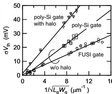
Fig. 3 Pelgrom plot ( $\sigma V_{th}$ ) for NMOS of several gate materials and halo implant.
