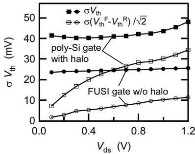
Fig. 5 Dependence of drain voltage ( $V_{\text{ds}}$ ) on  $\sigma V_{\text{th}}$  for SOTB NMOS.  $\sigma(V_{\text{th}}^{\text{F}} - V_{\text{th}}^{\text{R}})/\sqrt{2}$  is shown.
