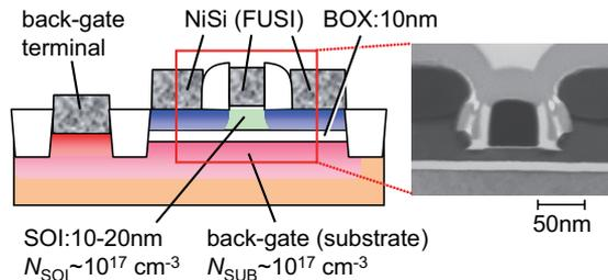
Fig. 1 Schematic cross-section of SOTB transistor. Features: (i) Small  $\sigma V_{th}$  due to low  $N_{SOI}$ , (ii) Excellent short-channel-effect immunity due to thin SOI and BOX, (iii) Back-gate bias control capable of trimming  $V_{th}$  and performance boosting. (iv) I/O bulk transistors can be integrated.
