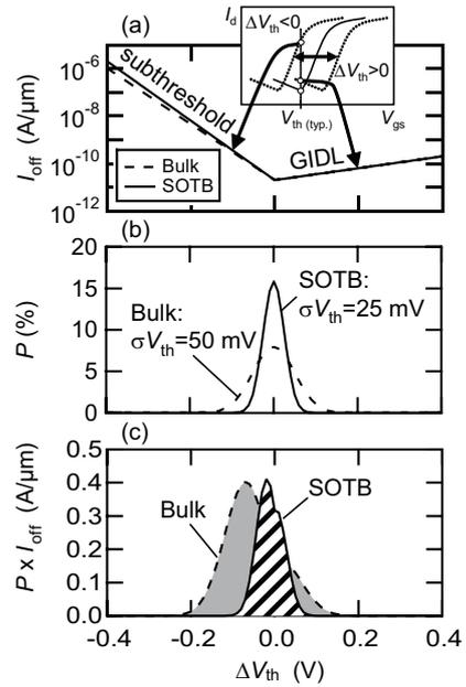
Fig. 6 Estimation of leakage current reduction by decreasing  $\sigma V_{\text{th}}$ . (a)  $I_{\text{off}}$  versus  $\Delta V_{\text{th}}$ . Inset indicates increase in  $I_{\text{off}}$  caused by change in  $V_{\text{th}}$  from the typical value. (b) Probability plot of  $V_{\text{th}}$ . (c) Expected value of  $I_{\text{off}}$ :  $P \times I_{\text{off}}$ .
