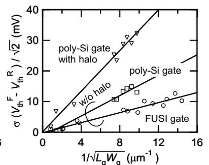
Fig. 4 Pelgrom plot ( $\sigma(V_{th}^F - V_{th}^R)/\sqrt{2}$ ): indicator of local variation) for same samples as in Fig. 3.
