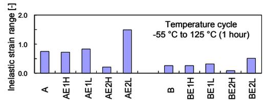
Fig. 5 Inelastic strain ranges of the solder bump in a temperature cycle of -55°C to 125°C
