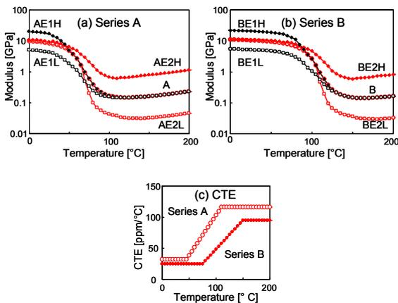
Fig. 2 Physical properties of underfills used in analyses: (a) Series A modulus, (b) Series B modulus, and (c) CTE
