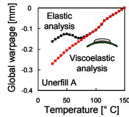
Fig. 3 Comparison of global warpage between analysis methods
