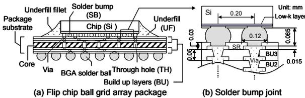
Fig. 1 Structures of the flip chip package and solder bump joint used in analyses
