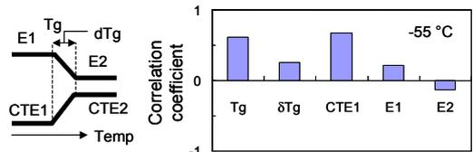
Fig. 6 Correlation coefficient between the energy release rate at the tip of the delamination crack of a low- $k$  layer and the factor of underfill properties at -55°C.
