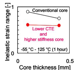
Fig. 8 Calculated inelastic strain ranges of a solder bump for FC-BGA packages with a thin substrate
