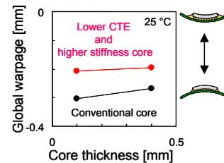
Fig. 7 Calculated warpage for FC-BGA packages with a thin substrate
