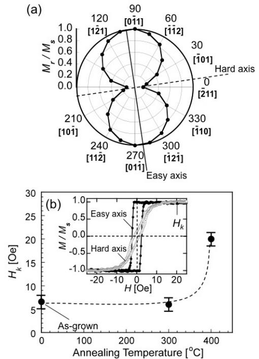
**Fig. 3.** (a) The polar plot of remanent magnetization normalized by saturation magnetization for the  $\text{Fe}_3\text{Si}$  layer annealed at  $400^\circ\text{C}$  for 30 min. (b) Anisotropy field as a function of annealing temperature (annealing time : 30 min). The inset shows normalized magnetization curves for the sample annealed at  $400^\circ\text{C}$  for 30 min.
