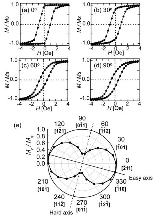
**Fig. 2.** Normalized magnetization curves of the as-grown  $\text{Fe}_3\text{Si}$  epilayer for field directions of  $\alpha =$  (a)  $0^\circ$ , (b)  $30^\circ$ , (c)  $60^\circ$ , and (d)  $90^\circ$ . (e) The polar plot of normalized remanent magnetization. The magnetic easy and hard axes are denoted as the solid and dashed lines, respectively.
