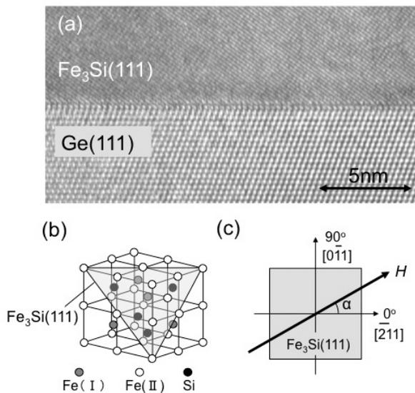
**Fig. 1.** (a) Cross-sectional TEM micrograph of an as-grown  $\text{Fe}_3\text{Si}/\text{Ge}(111)$ . (b) Schematic diagram of the  $\text{DO}_3$  unit cell of the  $\text{Fe}_3\text{Si}$ . (c) Definition of the direction of external magnetic fields ( $H$ ) applied in the film plane.
