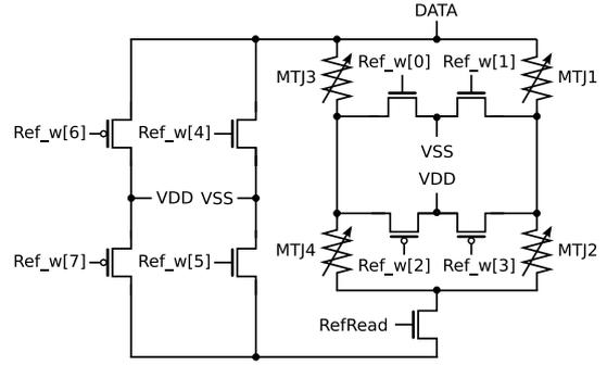
Fig. 5. SPRAM reference cell circuitry.
