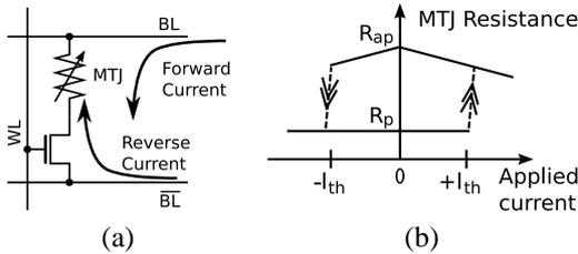
Fig. 3. (a) SPRAM cell circuitry and (b) its I-R characteristic ( $R_p = 1 \text{ k}\Omega$ ,  $R_{ap} = 3 \text{ k}\Omega$ ,  $I_{th} = 200 \mu\text{A}$ ).
