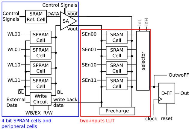
Fig. 2. Block diagram of two-inputs logic block with SPRAM.
