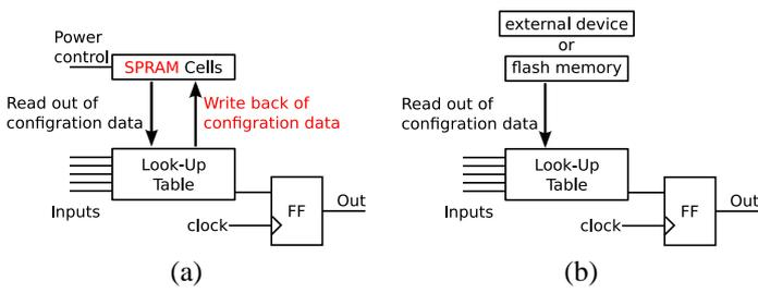
Fig. 1. Comparison of improved logic block with conventional one: (a) SPRAM-based FPGA; (b) conventional FPGA.
