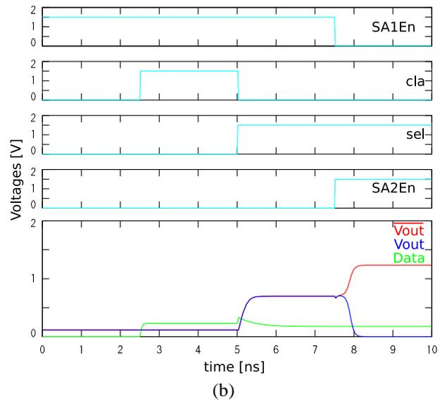
Fig. 6. Simulation results with clock frequency is 200 MHz and power supply is an 1.5-V: (a) time series of two-inputs LUT and D-FF simulation with MTJ is 3 kΩ (logical "1"); (b) time series of SA simulation with MTJ is 3 kΩ (logical "0").
