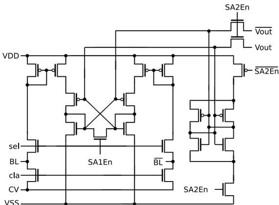
Fig. 4. Sense amplifier circuitry.
