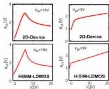
Fig. 4. Potential values at the channel/drift junction  $\phi_{sd1}$  as a function of gate voltage  $V_g$  and drain voltage  $V_d$  in comparison to 2D-device simulation results.
