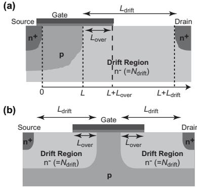
Fig. 1. Cross-sections of the LDMOS (a) and HVMOS (b) high-voltage MOSFET devices.
