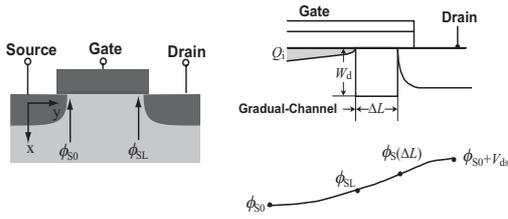
Fig.2. Important surface potentials calculated in HiSIM2 for the bulk MOSFET.
