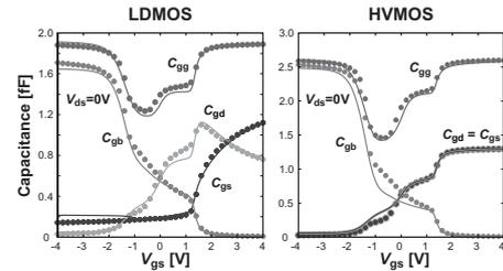
Fig. 7. Capacitances calculated for the LDMOS and symmetric HV-MOS structures with HiSIM-HV (lines) and 2D-device simulation (symbols).
