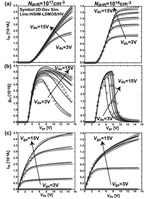
Fig. 5.  $I-V$  and  $g_m$  comparison between 2D-device simulator (symbols) and HiSIM-HV (lines) for the LDMOS structure with different drift-region doping of  $10^{17}\text{cm}^{-3}$  (left) and  $10^{16}\text{cm}^{-3}$  (right).
