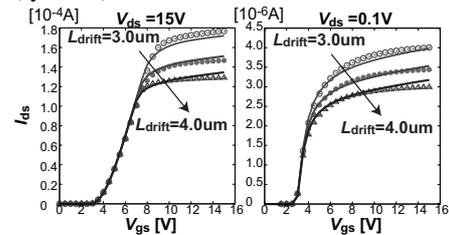
Fig. 8. Scalability of HiSIM-HV with drift-region length  $L_{drift}$ . The plots show the  $I_{ds}-V_{gs}$  characteristics at high and low drain bias in comparison of 2D-device simulation and HiSIM-HV results.
