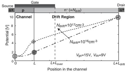
Fig. 3. Calculated potential distribution along the channel with HiSIM-HV (shown with symbols) for two  $N_{drift}$  concentrations.
