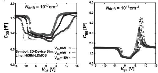
Fig. 6.  $C_{gg}$ -capacitance comparison between 2D-device simulation (symbols) and HiSIM-HV (lines) for the LDMOS structure with different drift-region dopings.
