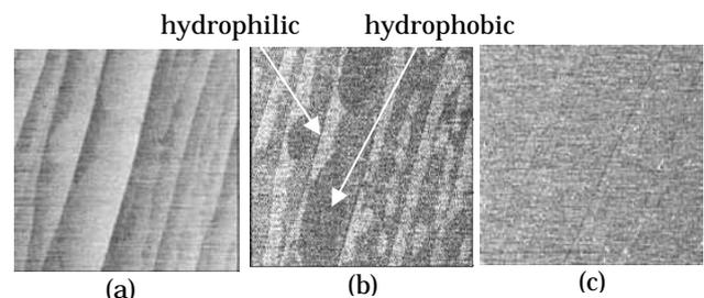
Fig. 1 AFM images on the sapphire surface. (a) Topographical and (b) frictional images of the acid-treated surface, and (c) frictional image of the thermally treated surface. Images are 15 x 15  $\mu\text{m}^2$ .
