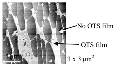
Fig. 2 OTS deposition pattern on an acid-treated surface.
