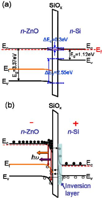
**Fig. 4** Energy band diagrams of the  $n\text{-ZnO}/\text{SiO}_x/n\text{-Si}$  LEDs.
