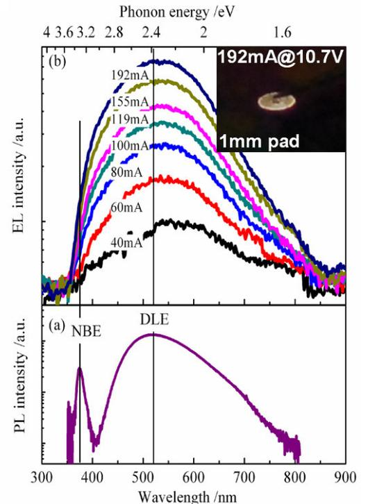
**Fig. 8** Room-temperature (a) PL, (b) EL of ZnO/MgO/TiN/Si heterostructured LEDs.
