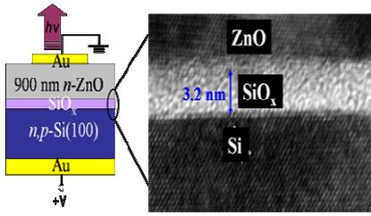
**Fig. 1** A schematic diagram of ZnO/Si heterostructured LEDs and its cross-sectional TEM image.
