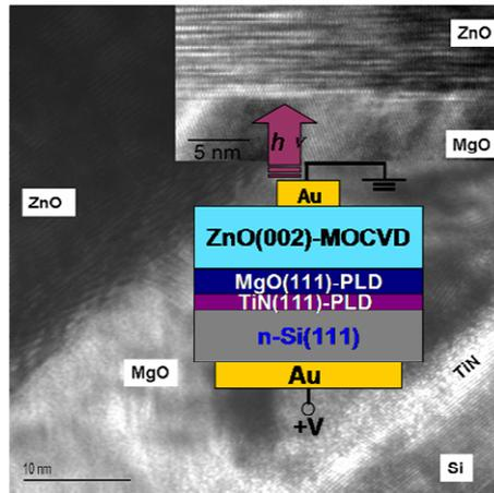
**Fig. 5** A schematic diagram of ZnO/MgO/TiN/Si heterostructured LEDs and its cross-sectional TEM.
