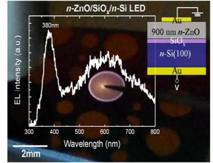
**Fig. 3** Room-temperature EL of the  $n\text{-ZnO}/\text{SiO}_x/n\text{-Si}$  LEDs.
