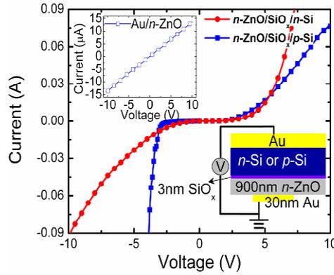
**Fig. 2** IV characteristics of ZnO/Si heterostructured diodes. Top inset shows the ohmic characteristic of Au/n-ZnO.
