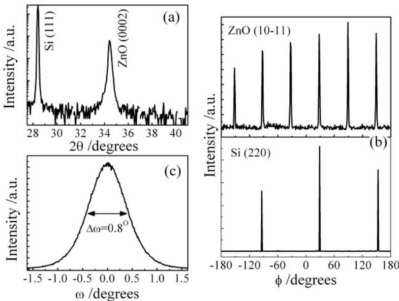
**Fig. 6** XRD spectrum of the epitaxial ZnO film on MgO/TiN buffered Si(111): (a)  $\theta/2\theta$  scan, (b)  $\Phi$ -scan for ZnO (10 $\bar{1}$ 1) and Si (220), and (c)  $\omega$ -scan rocking curve of ZnO (0002).
