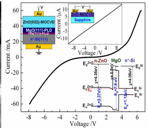
**Fig. 7** Typical IV characteristic of ZnO/MgO/TiN/Si heterostructured LEDs
