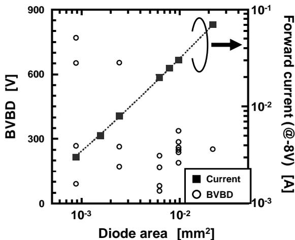
Figure 2. Maximum operation voltage ( $BV_{BD}$ ) and forward current (@-8V) of diamond pVSBD for various diode areas.
