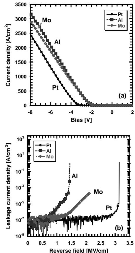
Figure 1(a) Forward and (b) reverse characteristics of diamond pVSBDs with various SBH.
