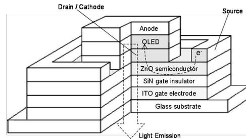
Fig.1 Structure of OLET using thin-film ZnO films.
