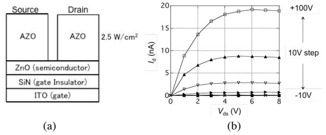
Fig.4 (a) Schematic of ZnO FET using AZO electrode deposited by uniform power deposition method and (b)  $I_d$ - $V_{ds}$  characteristics of ZnO FET.
