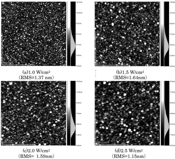
Fig. 3 Surface AFM morphologies of AZO films deposited at different rf power densities, (a)1.0 W/cm<sup>2</sup>, (b)1.5 W/cm<sup>2</sup>, (c)2.0 W/cm<sup>2</sup>, (d)2.5 W/cm<sup>2</sup>.
