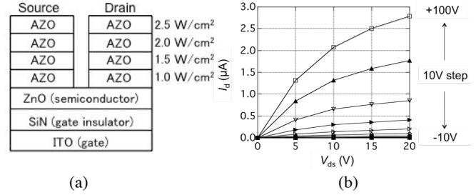
Fig. 5 (a) Schematic of ZnO FET using AZO electrode deposited by stepped power deposition method and (b)  $I_d$ - $V_{ds}$  characteristics of ZnO FET.
