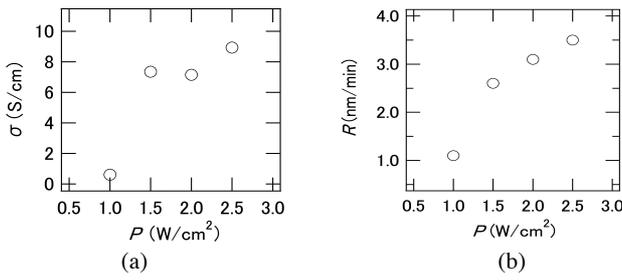
Fig. 2 (a) sheet resistance and (b) deposition rate as a functional of rf power.
