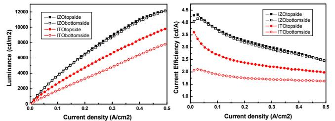
Fig. 3 (a) Luminance and (b) current efficiency vs current density curves with the IZO and ITO cathode.
