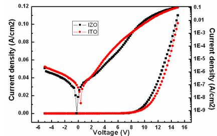
Fig. 2 J-V characteristics of FTPLD deposited with the IZO and ITO cathode.
