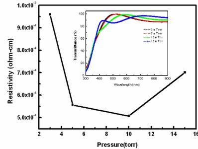
Fig. 1 The resistivity of IZO which were deposited under different working pressure. The insert shows the transmittance of IZO film deposited under different working pressure.
