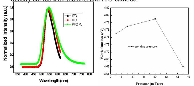
Fig. 4 EL characteristic for FTPLDs with IZO and ITO cathode and photoluminescence of the PFO film.
