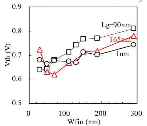
Fig. 10  $V_{th}$ - $W_{fin}$  characteristics of multi-FinFET NMOS with various  $L_g$ .
