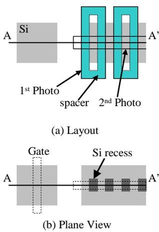
Fig. 3 (a) Layout of proposed scheme. Fin pitch and width are defined by 1<sup>st</sup> photo and spacer. Fin length is defined by 2<sup>nd</sup> photo. (b) Plane view after fin etching. A-A' corresponds to the vertical views in Fig. 2.
