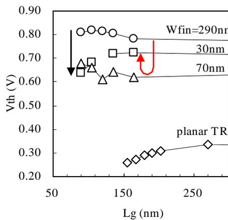
Fig. 9  $V_{th}$ - $L_g$  characteristics of multi-FinFET NMOS with various  $W_{fin}$ .
