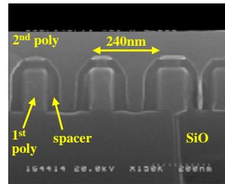
Fig. 5 A vertical SEM image after 2<sup>nd</sup> poly deposition.
