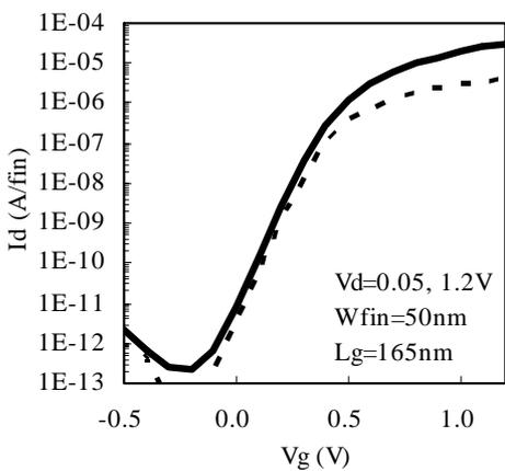
Fig. 8  $I_d$ - $V_g$  characteristics of multi-FinFET NMOS with TiN gate at 85C.
