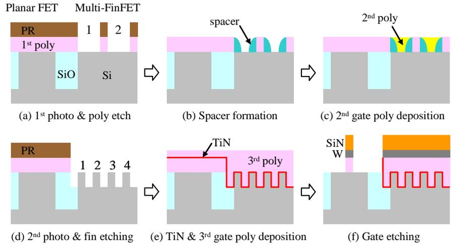
Fig. 2 The process flow of proposed spacer transfer multi-fin formation through the gate polysilicon layer.
