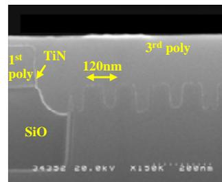
Fig. 6 A vertical SEM image after TiN and 3<sup>rd</sup> poly deposition.
