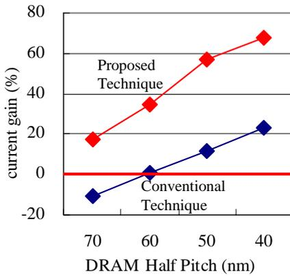
Fig. 4 Estimated drain current gain for a proposed technique and a conventional technique. Limitation of photo lithography, STI gap-filling and fin width consumption by cleaning and gate oxidation make large difference.
