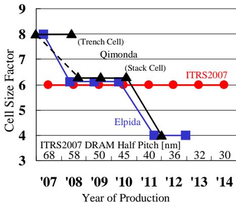
Fig. 1 Trend of DRAM cell scaling. Periphery shrink technology is strongly demanded according to reduction of cell size factor from 8 to 4.
