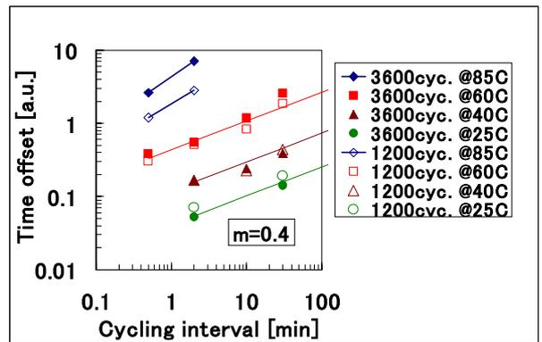
Fig.6 The time offset dependence on the cycling interval and temperature
