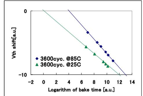
Fig.1 The cycling temperature dependence of Vt shift curve
