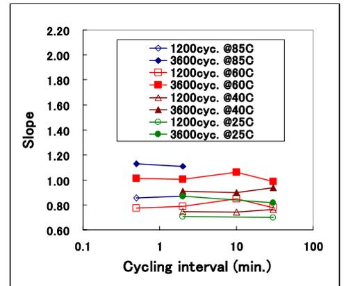
Fig.4 The cycling interval dependence of the slope
