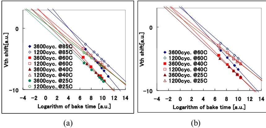
Fig.2 The dependence of Vt shift curve on the cycling numbers and temperature. The cycling intervals are 2min.(a) and 30min.(b).
