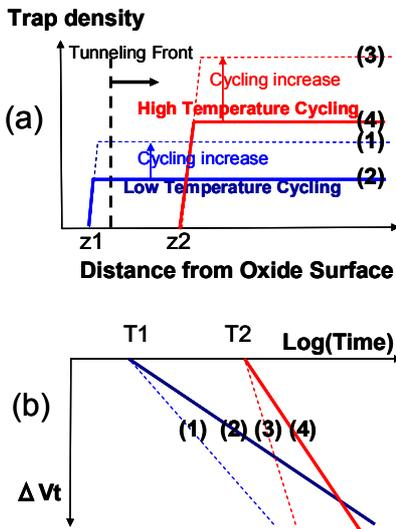
Fig.3 The tunneling Front Model
