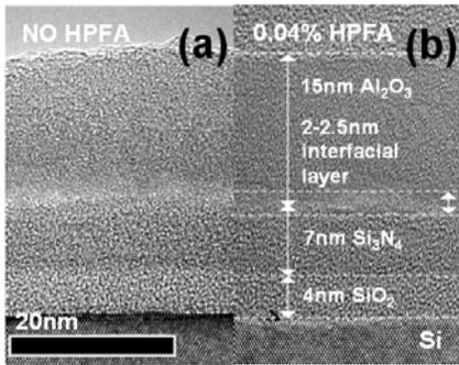
Fig. 3 Cross-sectional TEM images (a) NO HPFA sample (b) 0.04 % HPFA sample
