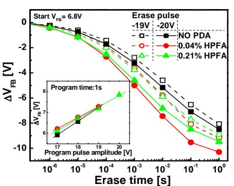
Fig. 8 The program (inset) and erase speed characteristics after 0.04 % and 0.21 % HPFA
