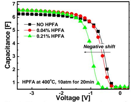
Fig. 2 The change of the capacitance of MANOS devices after 0.04 % and 0.21 % HPFA
