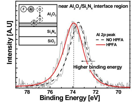
Fig. 5 XPS spectra of Al 2p near the Al<sub>2</sub>O<sub>3</sub>/Si<sub>3</sub>N<sub>4</sub> interface region and a physical model of fluorine passivation
