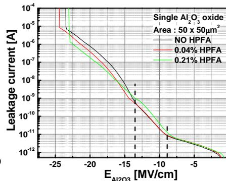
Fig. 7 The leakage current of single Al<sub>2</sub>O<sub>3</sub> MIS capacitors after 0.04 % and 0.21 % HPFA
