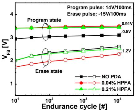
Fig. 9 Endurance cycle characteristics of NO HPFA, 0.04 % and 0.21 % HPFA samples
