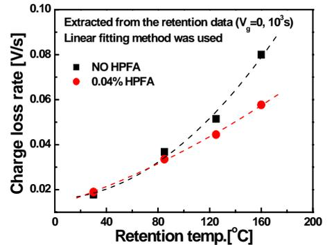
Fig. 11 The charge loss rates as a function of temperature of NO HPFA and 0.04 % HPFA samples
