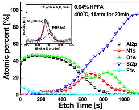
Fig. 4 XPS depth profile analysis and XPS spectra of F 1s in Al<sub>2</sub>O<sub>3</sub> after 0.04 % HPFA (inset figure)
