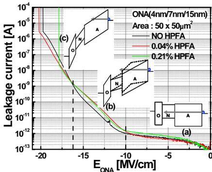
Fig. 6 The leakage current of MANOS devices after 0.04 % and 0.21 % HPFA and corresponding energy band diagrams
