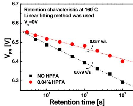
Fig. 10 The retention characteristics of NO HPFA and 0.04 % HPFA samples at 160 °C
