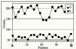
Fig. 2 The scanning profiles of an EDX spectroscopy at the ATE Ir/ $\text{IrO}_2$  /TE Ir layer from A to B in Fig. 1(b).
