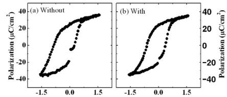
Fig. 5  $P-V$  hysteresis loops of the edge cell (a) without and (b) with dummy cells applied.
