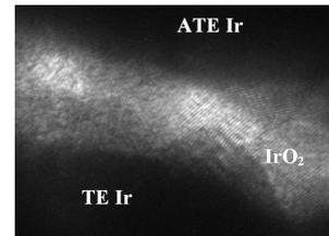
Fig. 6 A STEM image at the  $\text{IrO}_2$  interface between ATE Ir and TE Ir after the HTS and HTOL test.
