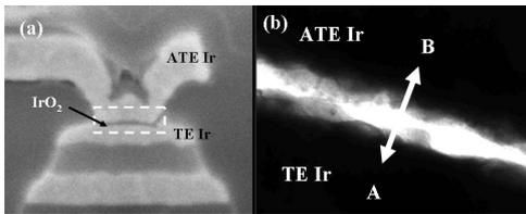
Fig. 1 (a) Micrographs of the failed cell capacitor after an HTS test during 500 hours in package-level and (b) a STEM image of the dashed rectangle in Fig. 1(a).
