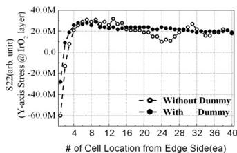
Fig. 4 Stress projected on the  $\text{IrO}_2$  layer as a function of the number of memory cells located from the edge boundary.
