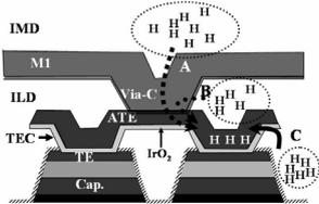
Fig. 3 The possible diffusion paths of atomic hydrogen for a path 'A' arising from forming-gas anneal processes, for a path 'B' resulted from ILD processes after the ATE formation, and for a path 'C' due to ILD processes after formation of the cell capacitors .
