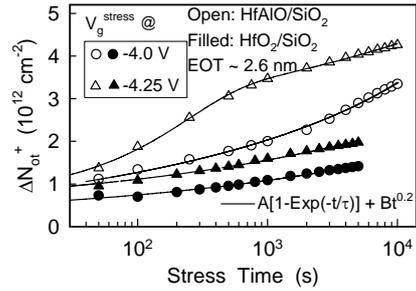
Fig. 4 Area density of oxide trapped charges as a function of stress time in HfAlO/SiO<sub>2</sub> (open) and HfO<sub>2</sub>/SiO<sub>2</sub> (solid) stacks with stress voltage as a parameter.
