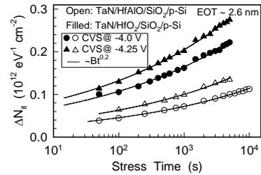
Fig. 5 Area density of stress-induced interface states as a function of stress time in HfAlO/SiO<sub>2</sub> (open) and HfO<sub>2</sub>/SiO<sub>2</sub> (solid) stacks with stress voltage as a parameter.
