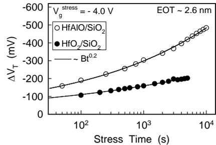
Fig. 6 Threshold voltage shift relative to the fresh device as a function of stress time in HfAlO/SiO<sub>2</sub> (open) and HfO<sub>2</sub>/SiO<sub>2</sub> (solid) stacks during CVS at -4.0 V.
