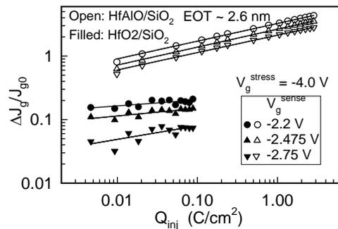
Fig. 7 Normalized SILC as a function of injected electron fluence in HfAlO/SiO<sub>2</sub> (open) and HfO<sub>2</sub>/SiO<sub>2</sub> (solid) stacks after CVS at -4.0 V with sensing voltage as a parameter.
