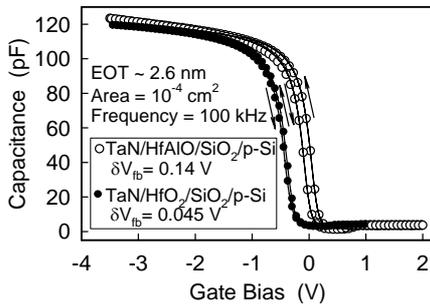
Fig. 1 Bi-directional C-V plot in fresh devices with HfAlO/SiO<sub>2</sub> (open) and HfO<sub>2</sub>/SiO<sub>2</sub> (solid) stacks. Curves are from QM simulation.
