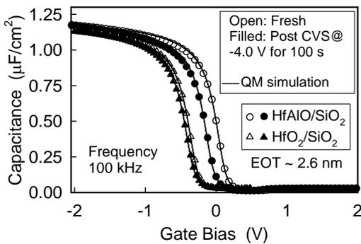
Fig. 3 High-frequency C-V curves recorded before and after CVS at -4.0 V for 100 s with HfAlO/SiO<sub>2</sub> (circle) and HfO<sub>2</sub>/SiO<sub>2</sub> (triangle) stacks.
