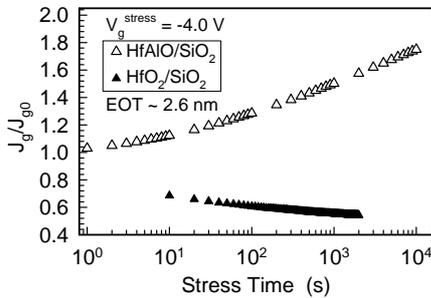
Fig. 2 Tunneling current density normalized to its initial value as a function of stress time during CVS at -4.0 V.
