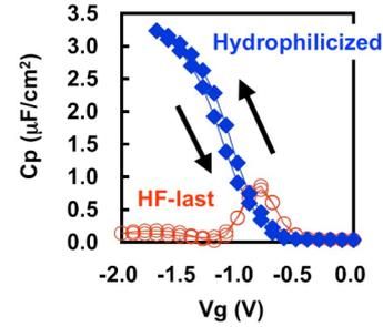
Fig. 2 Typical C-V characteristics of HfO<sub>2</sub>/Si direct-contact gate stacks fabricated on HF-last (open circle) and hydrophilicized surfaces (diamond). The HfO<sub>2</sub> cycles were set at 24 cycles.
