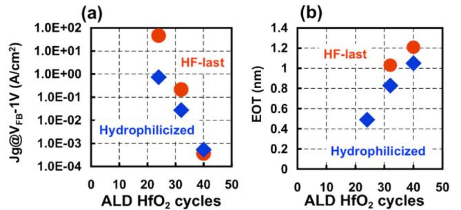
Fig. 3 Plots of (a) Jg vs ALD cycles and (b) EOT vs ALD cycles of HfO<sub>2</sub>/Si direct-contact gate stacks fabricated on HF-treated (circle) and hydrophilicized (diamond) surfaces.
