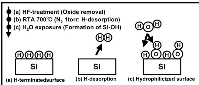
Fig. 1 Process flow and schematic models of surface hydrophilicization.
