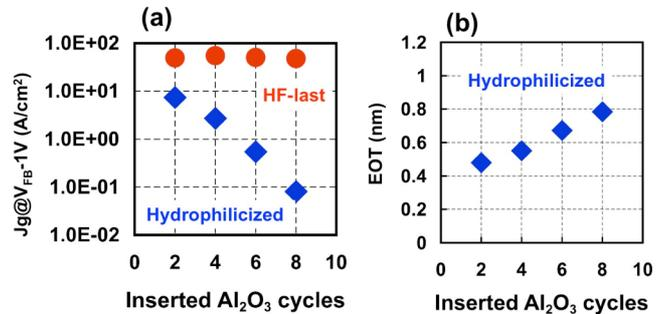
Fig. 5 Plots of (a) Jg vs ALD cycles and (b) EOT vs ALD cycles of ultra-thin Al<sub>2</sub>O<sub>3</sub> insertion layer for HfO<sub>2</sub>/Al<sub>2</sub>O<sub>3</sub>/Si direct-contact gate stacks fabricated on HF-treated (circle) and hydrophilicized (diamond) surfaces. HfO<sub>2</sub> cycles were set at 20 cycles.
