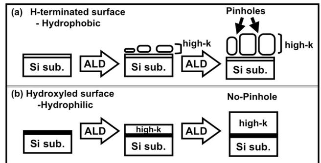
Fig. 4 Schematic models of ALD high-k/Si direct-contact gate stacks on (a) H-terminated and (b) hydrophilicized surfaces.
