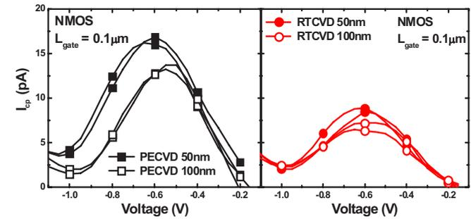
Fig 8. Comparison of  $I_{cp}$  with different CESL nitride. The RTCVD CESL devices exhibit lower charge pumping current than PECVD device which in turn lower interface charge trap density. In addition, both of PECVD and RTCVD devices decrease  $I_{cp}$  as thickness decrease.
