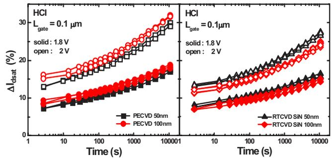
Fig 11. Comparison of  $\Delta I_{dsat}$  with different CESL nitrides. Under a high voltage stress, the thicker PECVD CESL device shows higher  $I_{dsat}$  degradation compared to 50nm PECVD CESL devices. However, in case of RTCVD, thicker devices exhibit lower  $I_{dsat}$  degradation.
