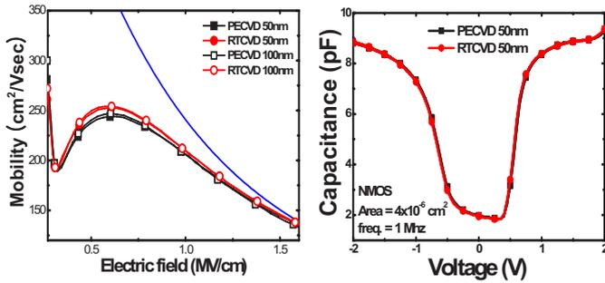
Fig 4. Mobility of NMOS with different CESL nitride. The RTCVD CESL devices show slightly higher mobility.
