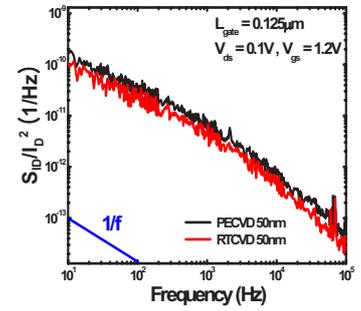
Fig 10. Low frequency noise measurement at  $V_{ds} = 0.1V$  and  $V_{gs} = 1.2V$  with PECVD and RTCVD CESL devices.
