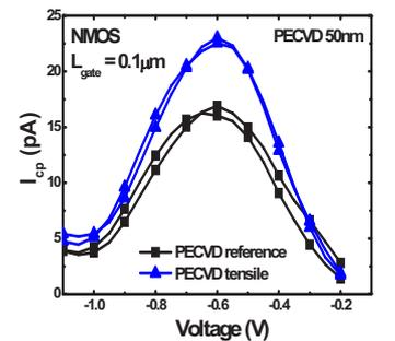
Fig 7. Comparison of  $I_{cp}$  with different PECVD CESL stressor nitride.  $I_{cp}$  in the PECVD tensile stressor devices was higher than in those with the reference nitride layers.
