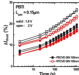
Fig 12. Comparison of  $\Delta I_{dsat}$  in nMOS between PECVD and RTCVD CESL devices. The PECVD CESL devices show significant  $I_{dsat}$  degradation compared to RTCVD CESL devices.
