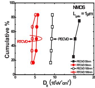
Fig 9. Comparison of  $D_{it}$  in gate length  $1 \mu m$  NMOS with different CESL elements. In long channel device, RTCVD samples also show lower interface charge trap density than PECVD samples
