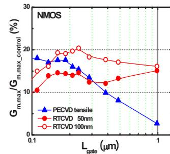
Fig 6. Comparison of  $G_{m,max} / G_{m,max,cont}$  between PECVD tensile CESL and RTCVD CESL devices. Unlike PECVD tensile CESL, the mobility improvement of RTCVD CESL was maximized around  $0.15 \sim 0.3 \mu m$
