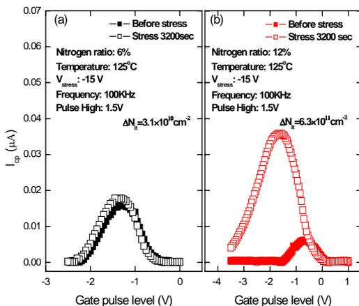
Fig. 10 Charge pumping current characteristic of Hf<sub>x</sub>Mo<sub>y</sub>N<sub>z</sub>/SiO<sub>2</sub> pMOSFET with N<sub>2</sub> ratio of 12%.
