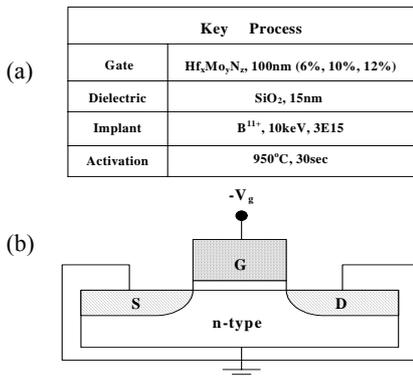
Fig.1 (a) The key process flow of Hf<sub>x</sub>Mo<sub>y</sub>N<sub>z</sub> metal gate pMOSFET device. (b) Bias configuration during NBTI stress.
