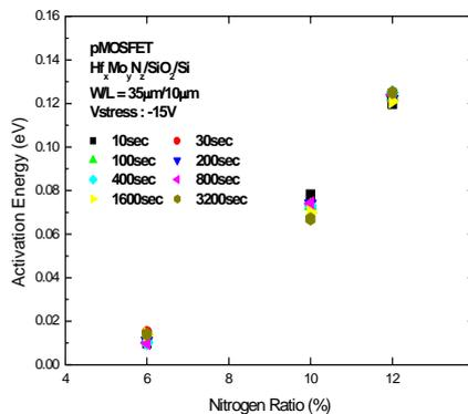
Fig. 8 Activation energy dependence of nitrogen ratio for Hf<sub>x</sub>Mo<sub>y</sub>N<sub>z</sub>/SiO<sub>2</sub> pMOSFET with -15 V, 3200 sec stress.
