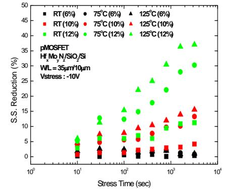
Fig. 6 NBTI stress time dependence of S.S. reduction for Hf<sub>x</sub>Mo<sub>y</sub>N<sub>z</sub>/SiO<sub>2</sub> pMOSFET with N<sub>2</sub> flow ratio of 12%.
