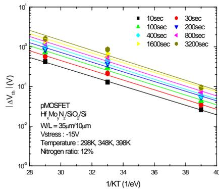
Fig. 7 Dependence of the  $V_{th}$  shift on the stress temperature for Hf<sub>x</sub>Mo<sub>y</sub>N<sub>z</sub>/SiO<sub>2</sub> pMOSFET with N<sub>2</sub> flow ratio of 12%
