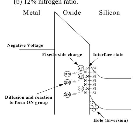
Fig. 12 Energy band diagram of the Hf<sub>x</sub>Mo<sub>y</sub>N<sub>z</sub>/SiO<sub>2</sub> pMOSFET during NBTI stress.
