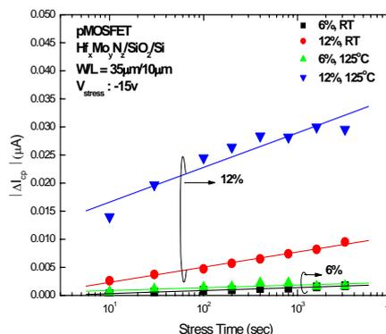
Fig. 11 Dependence of the  $\Delta I_{cp}$  on the stress time for Hf<sub>x</sub>Mo<sub>y</sub>N<sub>z</sub>/SiO<sub>2</sub> pMOSFET with N<sub>2</sub> ratio of 6% and 12%.
