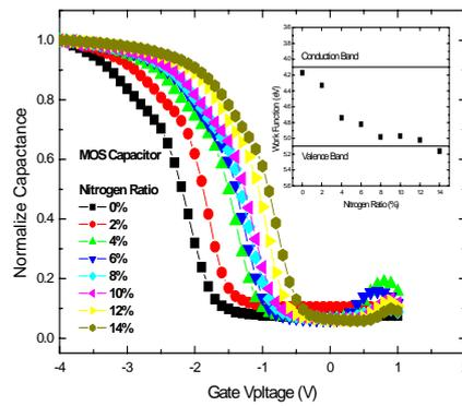
Fig.2 C-V characteristic of Hf<sub>x</sub>Mo<sub>y</sub>N<sub>z</sub>/SiO<sub>2</sub> capacitor. The Hf<sub>x</sub>Mo<sub>y</sub>N<sub>z</sub> gate electrode work function increased with increasing N<sub>2</sub> ratio.
