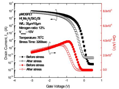
Fig.3 Typical transfer characteristic ( $I_{ds}$ - $V_{gs}$ ) of Hf<sub>x</sub>Mo<sub>y</sub>N<sub>z</sub>/SiO<sub>2</sub> pMOSFET with N<sub>2</sub> flow ratio of 12%.
