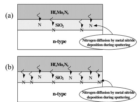
Fig. 9 Physical model for nitrogen atom distribution. The nitrogen diffuse into the SiO<sub>2</sub> during metal gate deposition. (a) 6% and (b) 12% nitrogen ratio.
