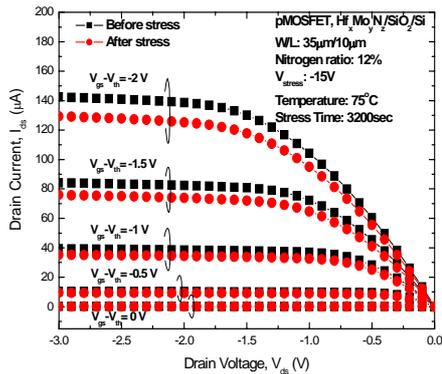
Fig.4 The output characteristic ( $I_{ds}$ - $V_{ds}$ ) of Hf<sub>x</sub>Mo<sub>y</sub>N<sub>z</sub>/SiO<sub>2</sub> pMOSFET with N<sub>2</sub> flow ratio of 12%.
