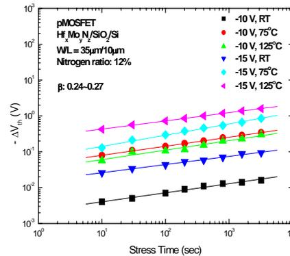
Fig. 5 NBTI stress time dependence of  $-\Delta V_{th}$  for Hf<sub>x</sub>Mo<sub>y</sub>N<sub>z</sub>/SiO<sub>2</sub> pMOSFET with N<sub>2</sub> flow ratio of 12%.
