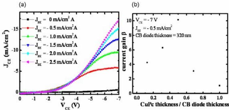
Fig. 2 (a) the collector-emitter current density ( $J_{CE}$ ) v.s collector-base voltage ( $V_{CE}$ ) at the base-emitter current density from 0 to -2.5  $\text{mA}/\text{cm}^2$  while the CuPc thickness / CB diode thickness ratio is 0.5 (b) the current gain as a function of CuPc thickness / CB diode thickness
