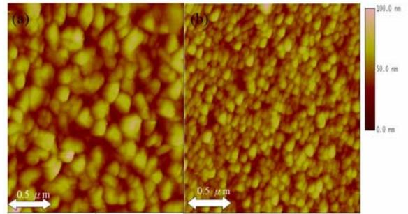
Fig. 3 the AFM images of 2.5 nm Al layer deposited on the CuPc thickness / CB diode thickness ratio of (a) 0.125 and (b) 1
