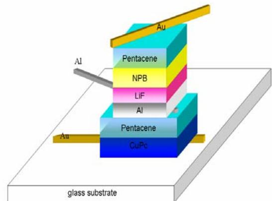
Fig. 1 the structure of the OBMT fabricated on the glass substrate.
