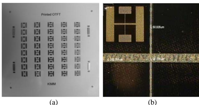
Fig. 2 Images of fabrication of roll printed OTFTs: (a) printed OTFT fabrication on the  $150\times 150$  mm plastic substrate and (b) with gate width  $W=57 \mu\text{m}$ , source and drain channel length  $L=27 \mu\text{m}$  (width  $W=202 \mu\text{m}$ ).
