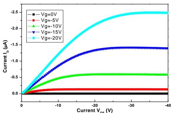
Fig. 4 Drain current  $I_{DS}$  versus drain voltage  $V_{DS}$  output characteristics of roll printed OTFT in the flexo printing
