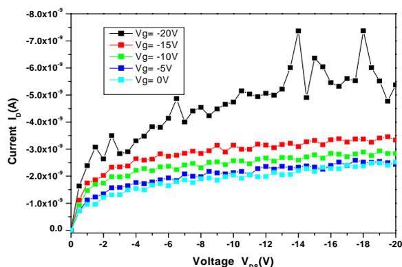
Fig. 3 Drain current  $I_{DS}$  versus drain voltage  $V_{DS}$  output characteristics of roll printed OTFT in the gravure printing
