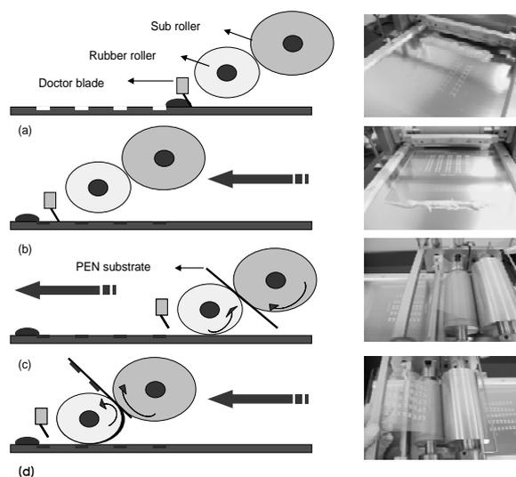
Fig. 1 Fabrication of printed electrodes in printed OTFTs using flexo printing: (a) pure Ag paste onto engrave plate (b) spread and inking on plate using doctor blade, (c) inserted plastic substrate between sub roll and rubber roll, and (d) roll printed electrode on plastic substrate.
