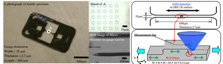
Fig.1 Photographs of SCS specimen and a schematic of line scan measurement.
