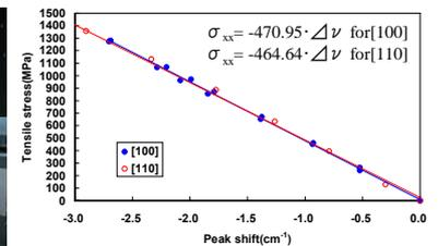
Fig.3 Relationship between Raman shift increment and applied tensile stress.
