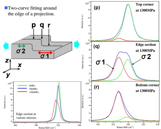
Fig.6 Raman spectra at the flat and edge sections.
