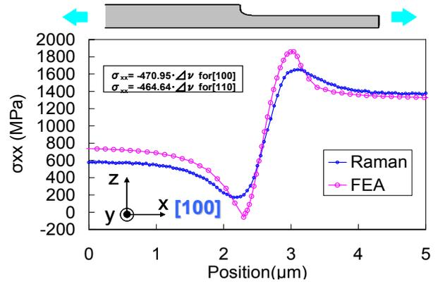
Fig.5 Tensile stress distribution obtained by one-curve fitting of Raman spectra and FEA.
