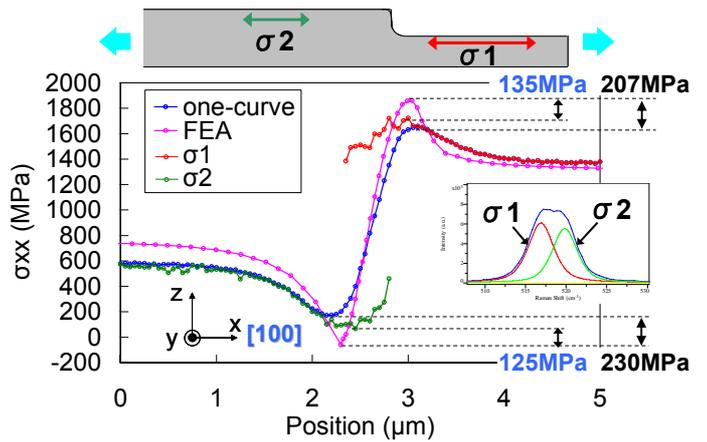
Fig.7 Stress distribution at the edge by two-curve fittings and FEA.
