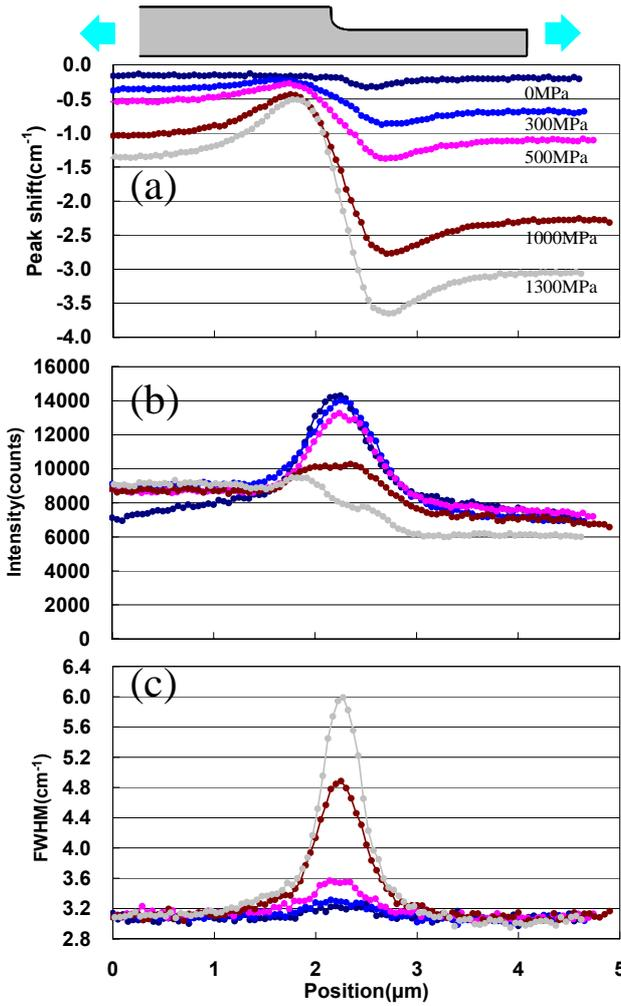
Fig.4 The peak shift, intensity, FWHM at the SCS convex structure when various tensile stress were applied.
