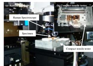
Fig.2 A Raman spectroscopic tensile test system.
