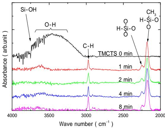
Fig. 5. FTIR spectra, in the range of 2000-4000cm<sup>-1</sup>
