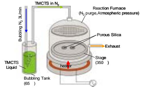
Fig. 2. Schematic diagram of a TMCTS annealing furnace
