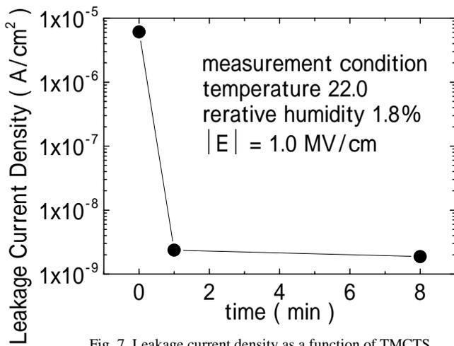
Fig. 7. Leakage current density as a function of TMCTS treatment time
