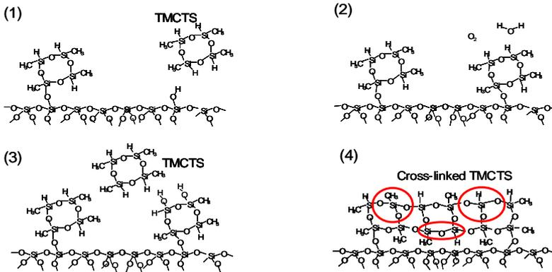
Fig. 3. Possible mechanism for TMCTS reaction on porous silica wall surface
