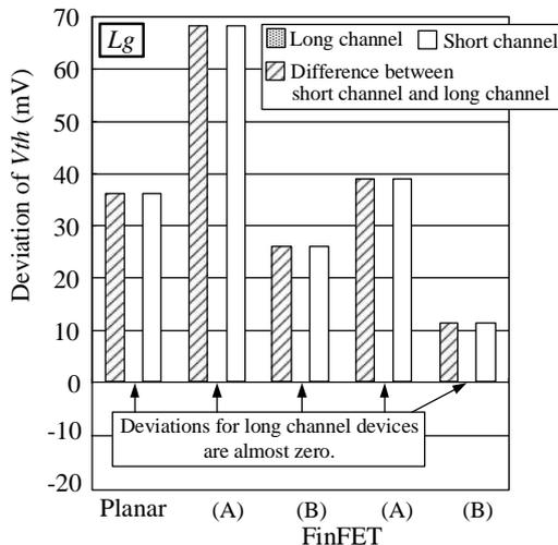
Fig.2  $V_{th}$  variations for 10% increase in  $L_g$ .
