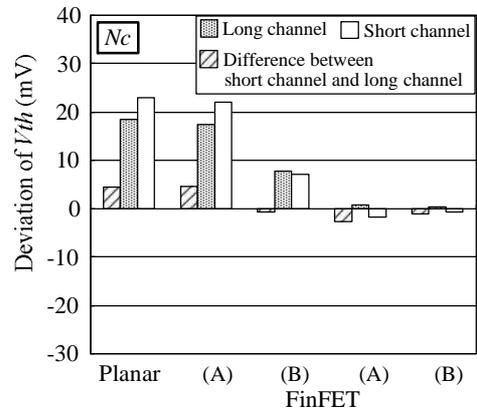
Fig.4  $V_{th}$  variations for 10% increase in  $N_c$ .
