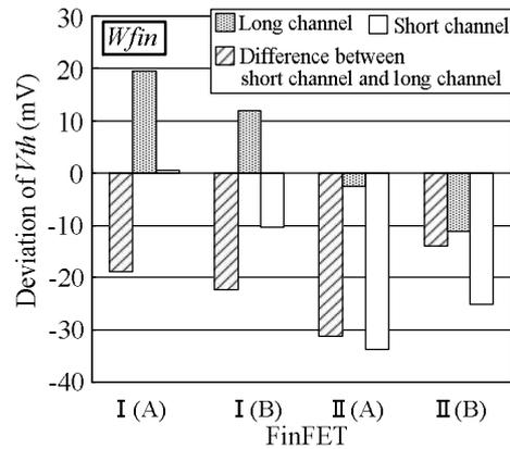
Fig.5  $V_{th}$  variations for 1.0 nm increase in  $W_{fin}$ .
