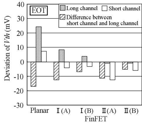
Fig.3  $V_{th}$  variations for 10% increase in EOT.
