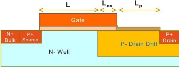
Fig. 1 Cross section of p-type DEMOS device used in this paper.
