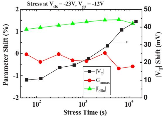
Fig. 3 Device parameter shift during hot-carrier stress.  $|V_T|$  and  $G_{max}$  are degraded.  $|I_{dlin}|$  is increased.
