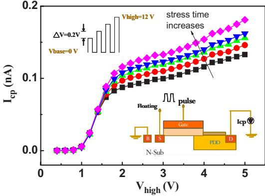
Fig. 5  $I_{cp}$  resulted from damage located in  $L_{ov}$  region. Significant  $\Delta N_{it}$  but small  $\Delta N_{ot}$  is created.
