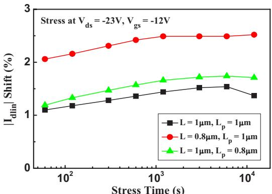
Fig. 8 Turnaround in  $|I_{dlin}|$  shift suggests that  $\Delta N_{it}$  in L and  $L_{ov}$  regions dominate device degradation as the stress time is longer.
