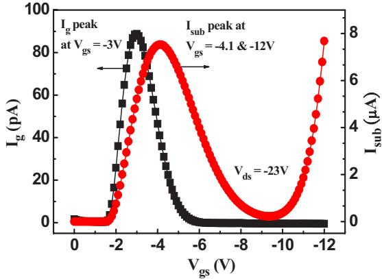
Fig. 2  $I_g$ - $V_{gs}$  and  $I_{sub}$ - $V_{gs}$  characteristics of p-type DEMOS device.  $I_g$ , 1st, and 2nd  $I_{sub}$  peaks occur at  $V_{gs} = -3V$ ,  $-4.1V$ , and  $-12V$ .
