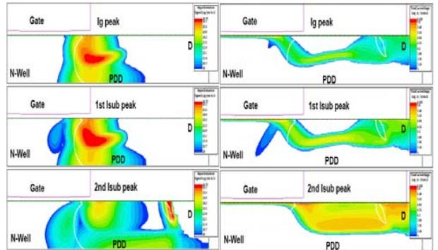
Fig. 6 Impact ionization (left) and current flow (right) when  $V_{gs}$  are biased under  $I_g$  peak, 1st, and 2nd  $I_{sub}$  peak conditions.
