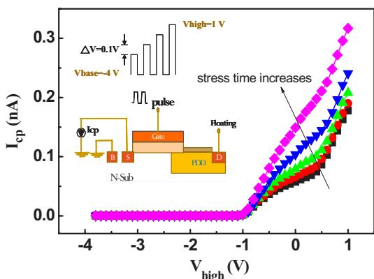
Fig. 4  $I_{cp}$  resulted from damage located in L region. Significant  $\Delta N_{it}$  but small  $\Delta N_{ot}$  is created.
