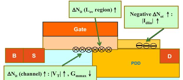
Fig. 7 Proposed two mechanisms for device degradation.  $\Delta N_{it}$  in channel region results in  $V_T$  and  $G_{max}$  degradation. Negative  $\Delta N_{ot}$  in  $L_p$  region results in  $|I_{dlin}|$  increase.
