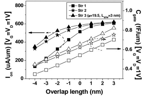
Fig.2 On-current and gate capacitance of nMOSFETs versus overlap length for various gate structures. For underlap cases, structure 2/3 show higher I<sub>on</sub>, but also suffer from higher capacitance.
