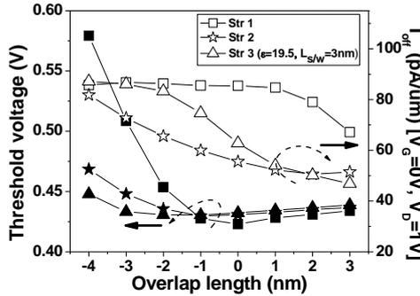
Fig.7 V<sub>th</sub> and I<sub>off</sub> versus overlap length for different gate structures. Lower leakages can be obtained in structure 2 and 3 due to better electrostatic control.
