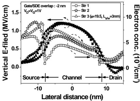
Fig.3 Profile of electron concentration at the surface of substrate for nMOSFET. More electrons are accumulated at the source region for structure 2/3 due to high vertical electric field.
