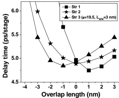
Fig.4 Delay time as a function of the overlap length (L<sub>ov</sub>). Each gate structure shows the minimum delay times at different L<sub>ov</sub> value.
