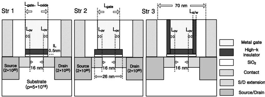
Fig.1 Schematic cross-sections of various gate structures. Structure 1 is conventional gate structure, which can be built by replacing polysilicon gate with metal gate. For structure 3, both polysilicon and gate dielectric are replaced by high-k/metal electrode, leading to high-k S/W MOSFET.
