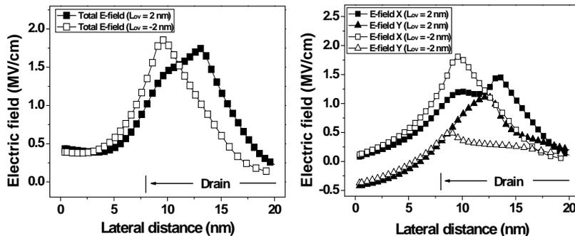
Fig.9 Electric fields for 2 nm S/D overlap and underlap structures. Maximum electric field can be located away from junction, leading to suppression of GIDL current.
