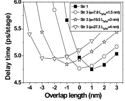
Fig.5 Delay time dependence on permittivity of gate dielectric layer in the structure 3. To meet same equivalent T<sub>ox</sub>, the physical thickness is adjusted.
