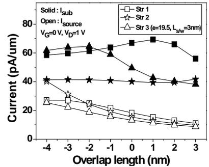
Fig.8 Subthreshold leakage and GIDL current versus overlap length. The leakage current is dominated by GIDL current instead of subthreshold leakage and affected by S/D overlap.
