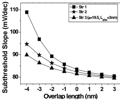
Fig.6 Subthreshold slope as a function of the overlap length. Better electrostatic control is achieved with high-k S/W MOSFET.
