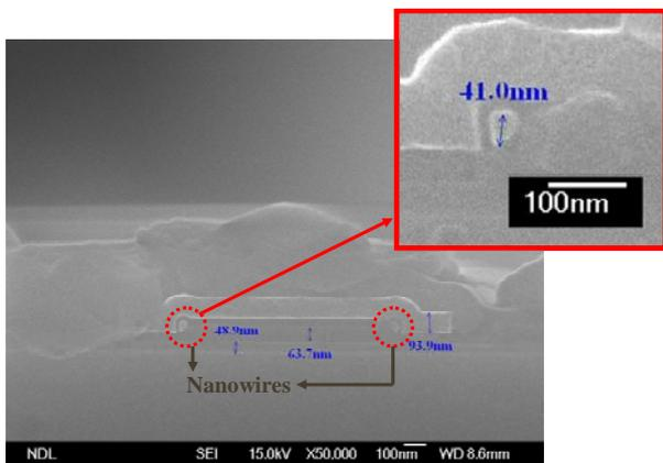
Fig. 3 SEM image of a fabricated S2 NWTFT.
