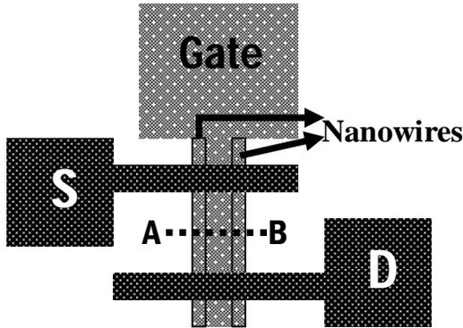
Fig. 1 Top view of the NW-TFT with inverse-T gate and top gate
