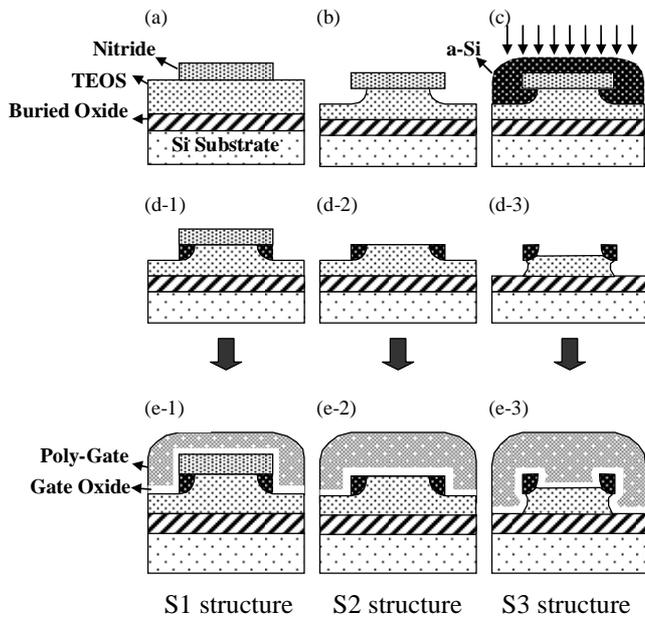
Fig. 2 Process sequence for forming three types of structures.
