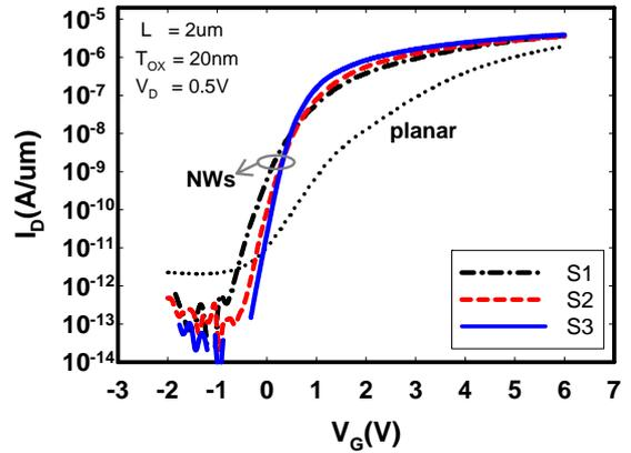
Fig. 4 Transfer characteristics of the planar and NW devices with channel length of 2 micron.
