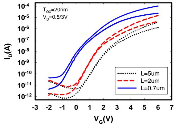
Fig. 5 Transfer characteristics of planar devices with channel length of 5, 2, and 0.7 micron.
