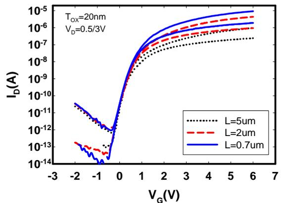
Fig. 6 Transfer characteristics of S3 NW devices with channel length of 5, 2, and 0.7 micron.
