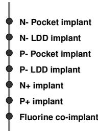
Fig.4 Fluorine co-implant process flow
