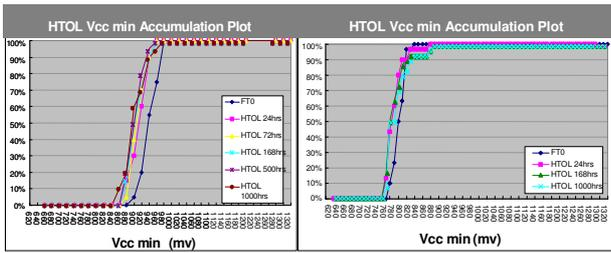
Fig.5 Vccmin drift accumulation plot ( 5a\_left : without Fluorine co-implant ) ( 5b\_right : with Fluorine co-implant)
