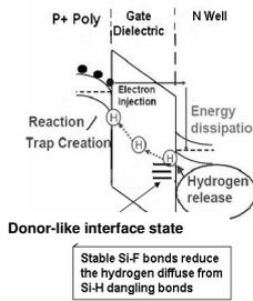
Fig.7 Energy band diagram of PMOS NBTI effect on Fluorine co-implant
