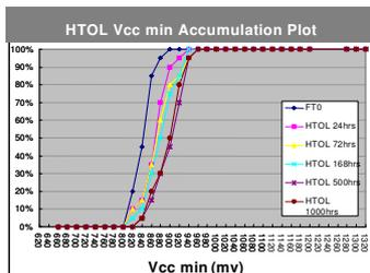
Fig.2 SRAM Vccmin drift after 125C, 1000hrs stress
