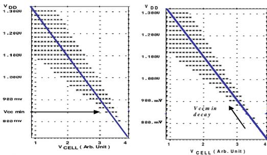
Fig.8 Vccmin shmoo ( left/right:non-stress/1000hrs stress )
