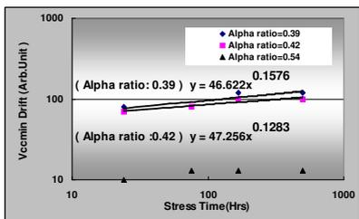
Fig.9 Vccmin drift with time dependence on alpha ratio split
