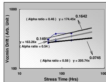
Fig.3 Vccmin drift with time dependence on different alpha ratio ( 0.46, 0.54, 0.58).
