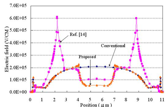
Fig. 2. The surface electric field distribution of the conventional, the device proposed in [14] and the proposed structure.
