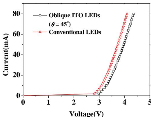
Fig. 5 Current-voltage characteristics of oblique ITO LEDs and conventional LEDs.
