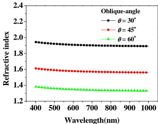
Fig. 3 The dependence of refractive index on oblique-angle  $\theta$ .
