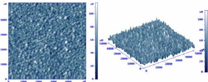
Fig. 4 AFM images of the oblique ITO nanorods array.
