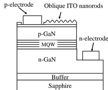
Fig. 2 Structure of ITO LEDs with oblique ITO nanorods.
