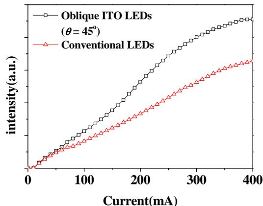
Fig. 6 Output light intensity of oblique ITO LEDs and conventional LEDs.
