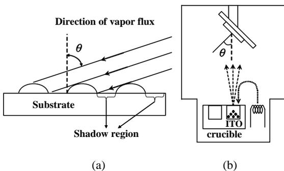
Fig. 1 (a) Schematic of oblique deposition and (b) Oblique e-beam deposition system.
