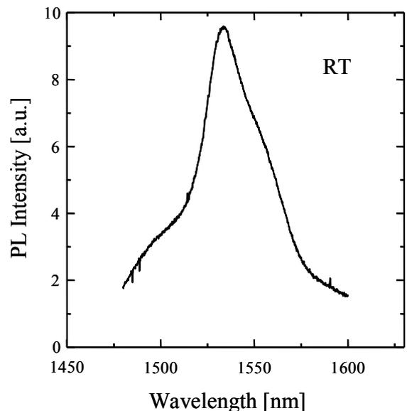
Fig. 1. Room-temperature photoluminescence spectrum of Er-doped  $\text{SnO}_x$  annealed at 700°C.
