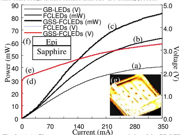
Fig. 3 (a)-(e) The corresponding L-I-V characteristics of the GB-LEDs, FCLEDs, and GSS-FCLEDs. (f) The schematic structure of GB-LEDs. (g) The photomicrographs view of GSS-FCLEDs.
