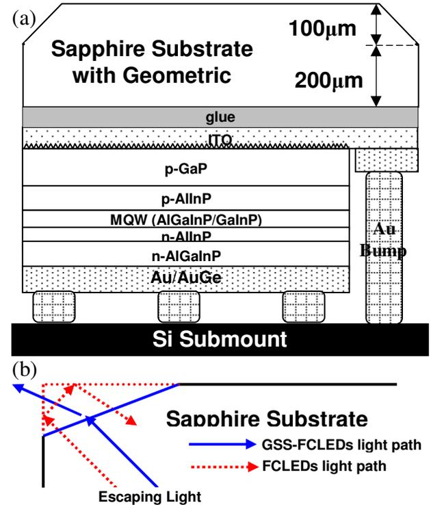
Fig. 1 (a) Schematic diagram of the AlGaInP-based GSS-FCLEDs structure with an oblique sapphire shaping sidewall were demonstrated by glue bonding. (b) Described with the different output light path of the novel GSS-FCLEDs and the oblique-free FCLEDs.
