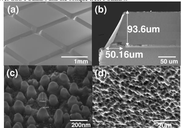
Fig. 2 SEM figures of (a) A top view of geometric sapphire shaping structure. (b) The cross section view of GSS-FCLEDs chip with an oblique sidewall. (c) Ni nano-mask clustered after RTA. (d) Nano-scale rough texture surface after ICP dry-etching process.
