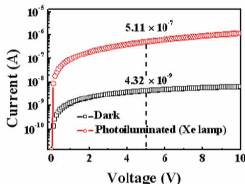
Fig. 4 I-V characteristics of ZnO photodetector measured in dark and under Xe illumination.
