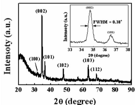
Fig. 3 XRD pattern of ZnO thin film.
