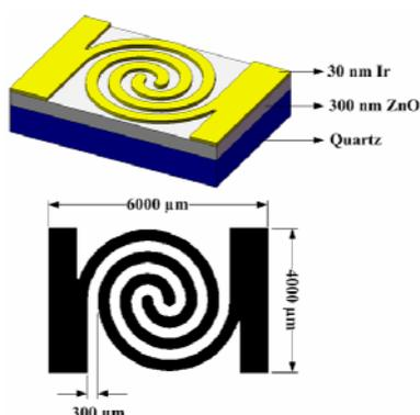
Fig. 1 The schematic structure of ZnO MSM photodetector.
