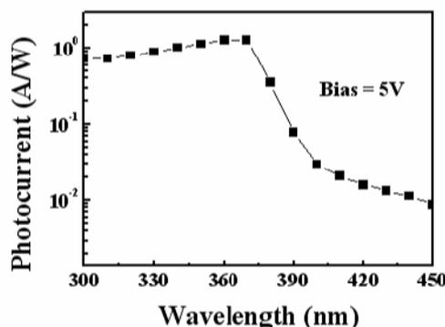
Fig. 5 The spectral response of the photocurrent measurement of ZnO MSM photodetector
