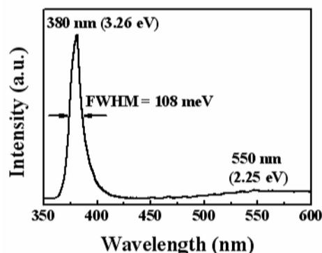
Fig. 2 The PL spectrum of ZnO thin film at room temperature.
