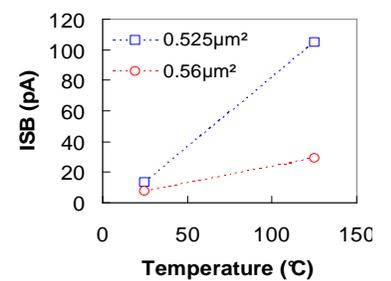
Fig.11: Isb at 25 and 125°C for 0.525µm² "Moore's like" bitcell and 0.56µm² "Large L" bitcell
