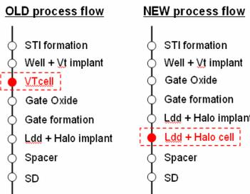
Fig.5: Process flow change for SRAM specific implants
