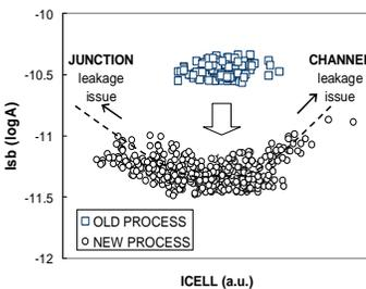
Fig.8: Isb=f(Icell) for OLD and NEW process
