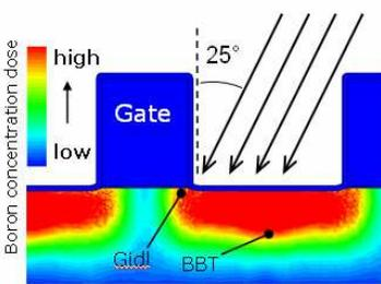
Fig.6: Implant scheme with low angle halos that not use gate shadowing, driving to high Gidl and S/D diode leakages
