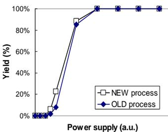
Fig.9: Yield at various Vdd power supply for OLD and NEW process
