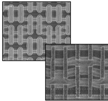
Fig.1: SEM top-view of 0.525µm² and 0.299µm² SRAM bitcell
