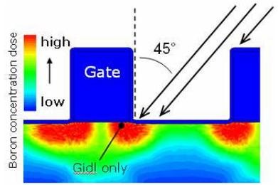
Fig.7: Implant scheme with high tilted halos that use the natural gate shadowing. In that case, S/D surfacic diode leakage is suppressed.
