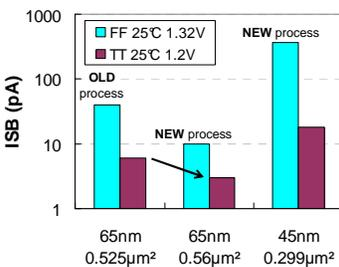
Fig.13: Isb of bitcells studied in this work in typical (TT) and process (FF) corners
