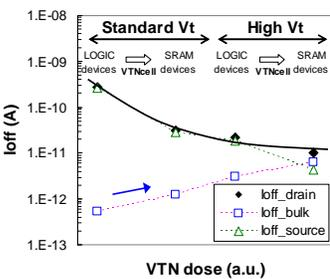
Fig.4: NMOS leakages for various channel doping level (with VTNcell implant before gate deposition)
