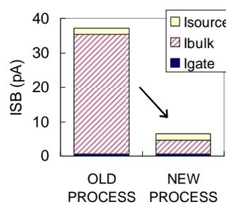
Fig.10: Comparison of Isb leakage components between old and new process flow in 65nm.
