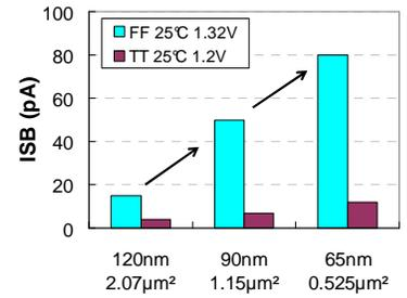
Fig.3: Isb of High-Density SRAM bitcells (with VTNcell implant before gate deposition)
