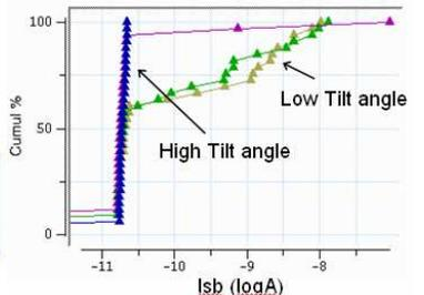
Fig.15: Isb measurements showing huge reduction of extrinsic leakages with high tilted pockets
