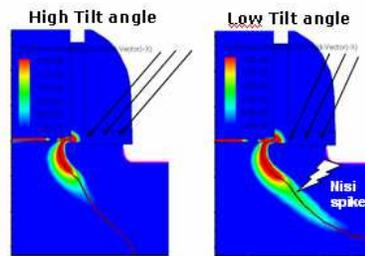
Fig.14: 2D TCAD simulations showing electric field at drain side for high (left) and low (right) tilt angles
