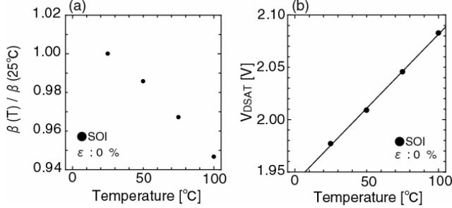
Fig. 4: (a) Temperature dependence on  $\beta$ . (b) Temperature dependence on  $V_{DSAT}$ .
