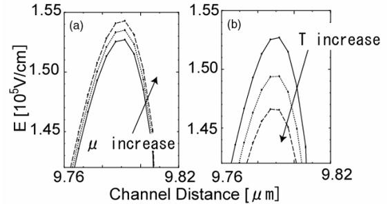
Fig. 6: Simulation results of variation of maximum electric field along the channel with carrier mobility (a) and device temperature (b). The results are consistent with experimentally observed variation in  $V_{DSAT}$ .
