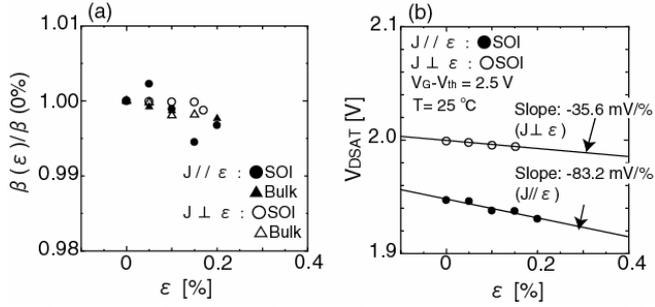
Fig. 3: (a) Uniaxial tensile strain dependence on  $\beta$ . (b) Uniaxial tensile strain dependence on  $V_{DSAT}$ .
