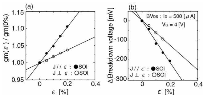
Fig. 2: Change with uniaxial tensile strain in transconductance  $g_m$  (a) and breakdown voltage (b) of an SOI MOSFET.
