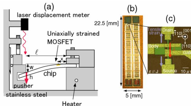
Fig. 1: (a) Schematic of cantilever bending tool constructed for the experiment which enables us to change temperature of the sample during application of strain. (b) Photo of an SOI chip containing MOSFETs. (c) Photomicrograph of a MOSFET in which twin-body was formed to reduce the body-tie resistance.
