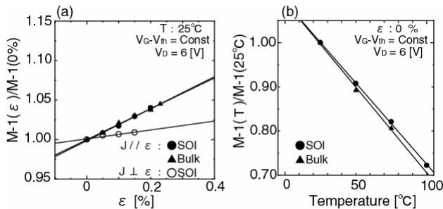
Fig. 5: (a) Dependence on uniaxial tensile strain of  $M-1$ . (b) Temperature dependence of  $M-1$ .  $M-1$  values were measured under constant  $V_G - V_{th}$  and  $V_D$ .
