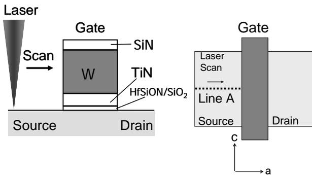
Fig.1 The sample structure used in the present work
