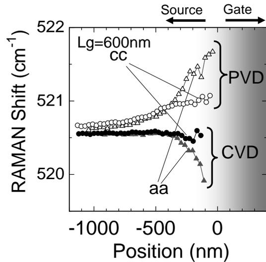
Fig.2 The spatial variation of the Raman shifts along line A in the S/D regions for PVD-W and CVD-W gates samples.
