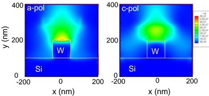
Fig.3 2D maps of the light intensity calculated with the FDTD simulations for the light sources of *a*-polarization and *c*-polarization.
