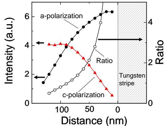
Fig.4 The light intensities at 5 nm below the Si channel surface for *a*- ( $\bullet$ ) and *c*-polarization ( $\blacktriangle$ ) light sources, and the ratios of the light intensity for *a*-polarization to that for *c*-polarization ( $\circ$ ) are plotted as a function of the probe distance from the gate edge.
