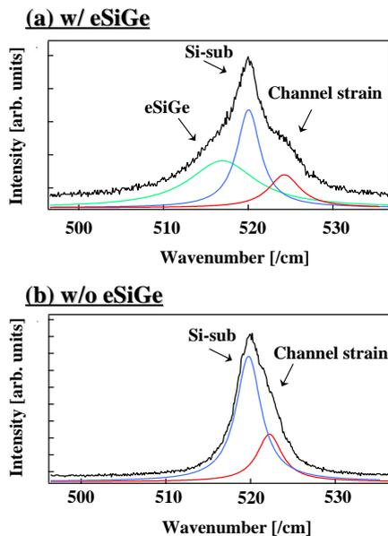
Fig. 4 Raman spectra obtained with 40-minute laser exposure from damascene-gate pFETs (a) with and (b) without eSiGe. Red, Blue, and Green lines signified the fitting line for each Peak.
