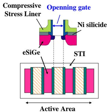
Fig. 1 Schematic diagram of damascene gate pFETs after dummy gate removal.
