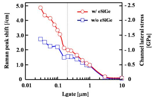
Fig. 5 Raman peak shift (left axis) and channel lateral stress (right axis) dependence on  $L_{gate}$  for pMOSFET with and without eSiGe.
