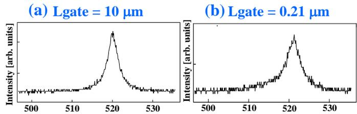
Fig. 2 Raman spectrum in the channel center obtained from (a)  $L_{gate} = 10 \mu\text{m}$  and (b)  $0.21 \mu\text{m}$ , respectively.
