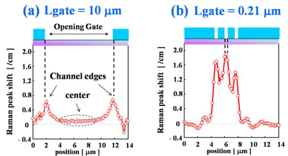
Fig. 3 Channel strain distribution obtained from (a)  $L_{gate} = 10 \mu\text{m}$  and (b)  $0.21 \mu\text{m}$ , respectively.
