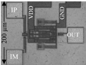
Fig.7. The chip micrograph.
