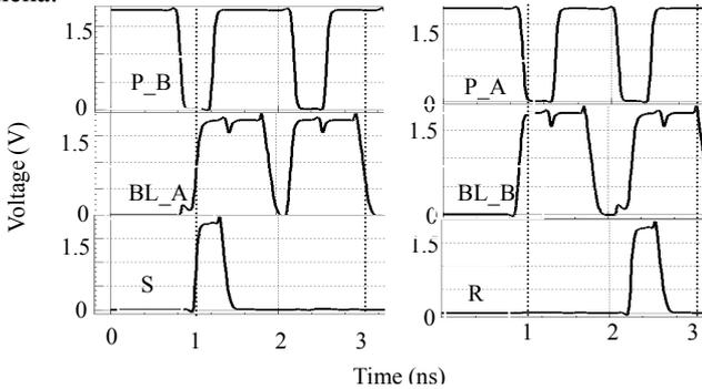
Fig.6(a). The controlled propagation mechanism. (a). Propagation through P\_B. (b). Propagation through P\_A.
