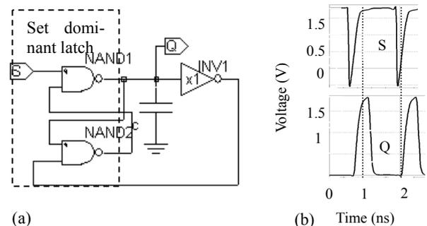
Fig. 3. The pulse widening circuit and simulation results. (a). Schematic diagram. (b). Response of the circuit.
