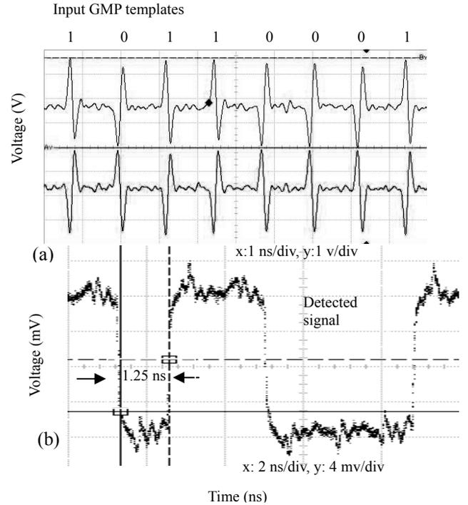
Fig. 9. The test result. (a). The input GMP templates of a random sequence of data. (b). The detected signal.
