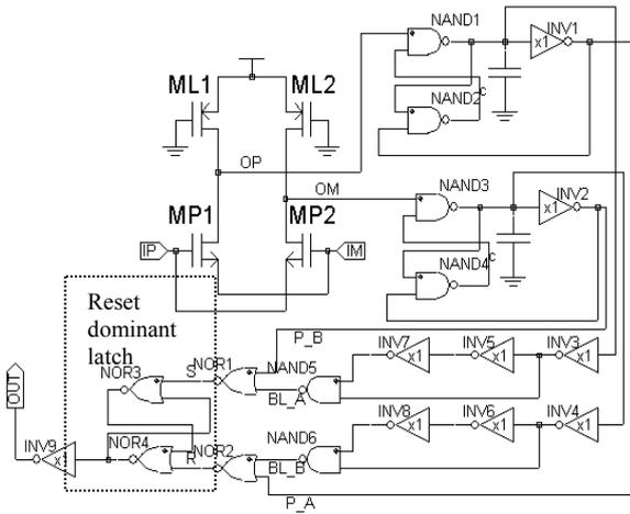
Fig.5. The overall schematic of the detector.
