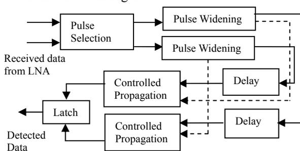
Fig. 1. Block diagram of the detector.
