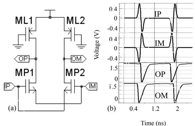
Fig. 2. The selector circuit and simulation results. (a). Schematic diagram. (b). Simulated waveforms.
